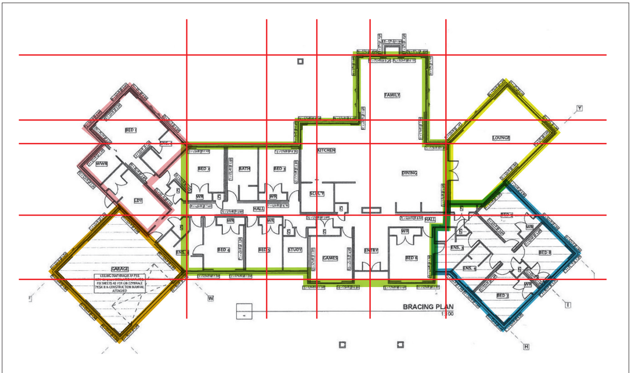
Figure 10. A building with a plan consisting of wings/blocks – bracing lines for the green block shown. Bracing capacity of walls common to both a wing and a block must be the sum of the requirements for the wing and the block.
