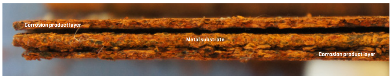
Figure 3. Corrosion products on the mild steel sample exposed at the wastewater treatment plant site for 1 year.
