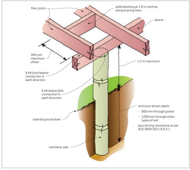
Figure 2. Cantilever piles.
