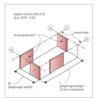
Figure 3. Bracing lines supporting diaphragms.
