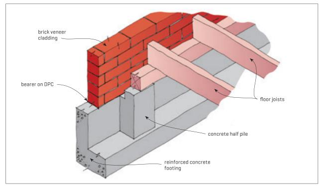
Figure 1. Suspended floor structure with semi-detached or half piles integrated into continuous foundation wall.
