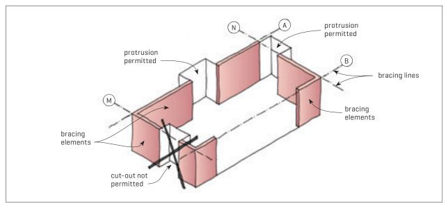
Figure 6. Ceiling diaphragm protrusions and cut-outs.
