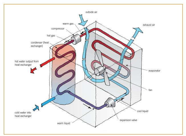
Figure 1. Air-source heat pump water heater cycle.
