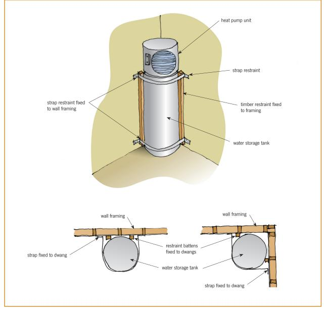
Figure 2. Recommended restraints from G12/AS1.
