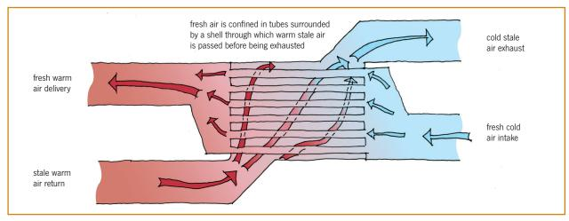
Figure 7. Principle of a counter-flow system.
