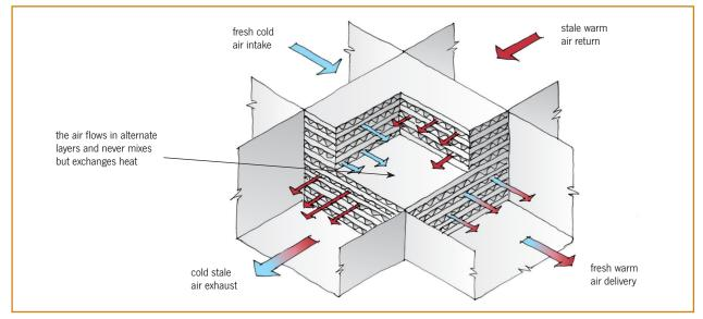
Figure 6. Principle of a cross-flow system.
