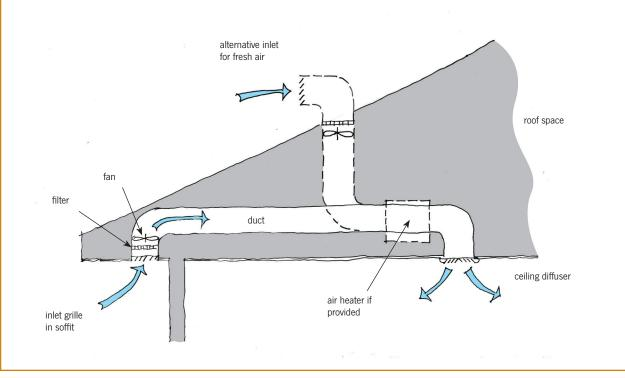
Figure 2. Mechanical ventilation supply-only system (also known as external air-sourced positive pressure ventilation system).
