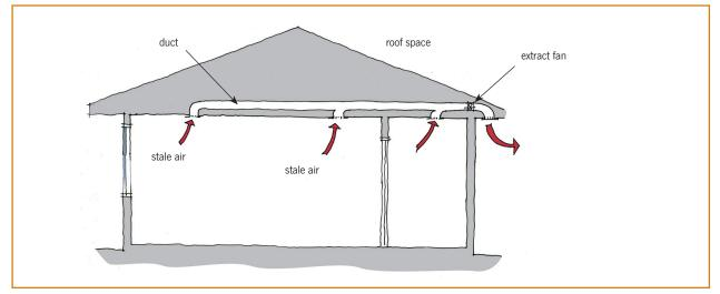
Figure 4. Mechanical ventilation general extract system.
