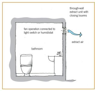
Figure 3. High flow rate localised extract system.
