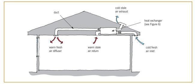
Figure 5. Mechanical ventilation heat recovery (MVHR) system.
