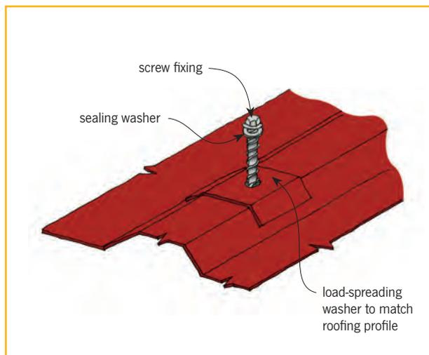
Figure 4. Load-spreading washer to metal roofing.
