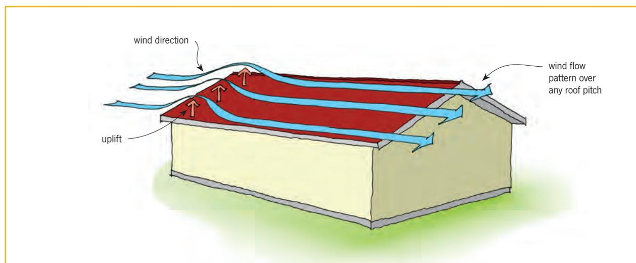
Figure 1. Wind parallel to ridge.
