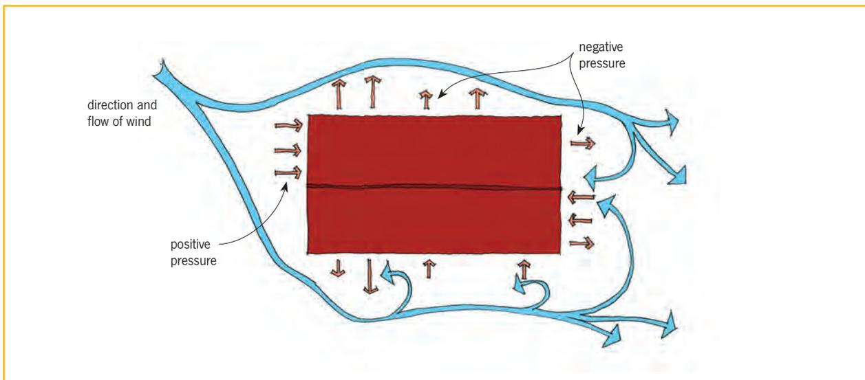
Figure 3. Wind pressure acting on walls.
