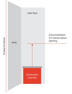
Figure 2. Schematic of BS 8414 test specimen
