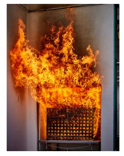
Figure 1. BS 8414 - combustion chamber
