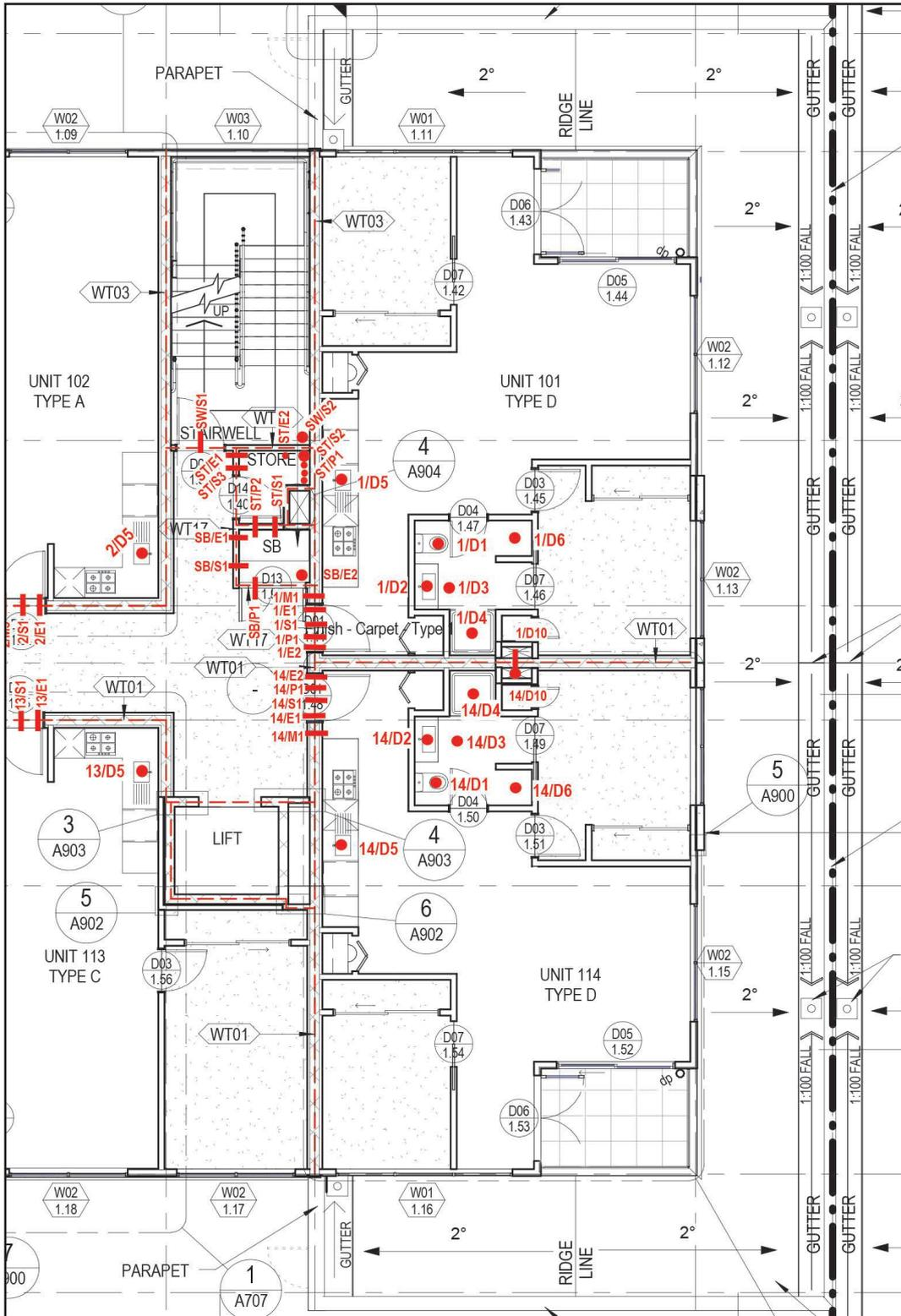
Figure 5. Example of plan of penetration seals
