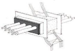
fire-rated polyurethane [PU] foam sheet
