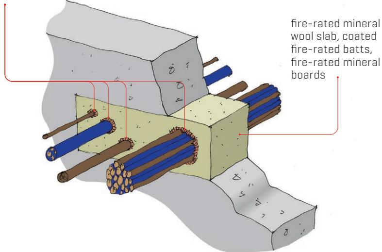
fire-rated mineral wool slab, coated fire-rated batts, fire-rated mineral boards
