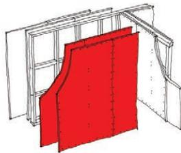
fire-rated plasterboard (applies to multi-layer and single layer walls; note that each manufacturer may colour their product differently)
