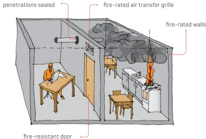
**Figure 2. Fire spread control using passive fire protection**
