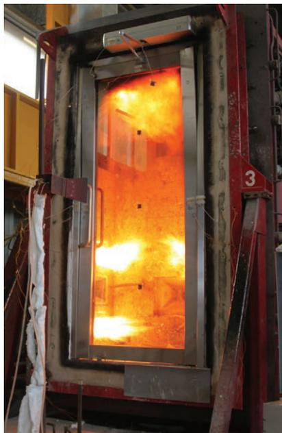
Pilot fire resistance furnace 2 m high × 1 m wide
