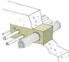
fire-rated mineral wool, slab board and blankets
