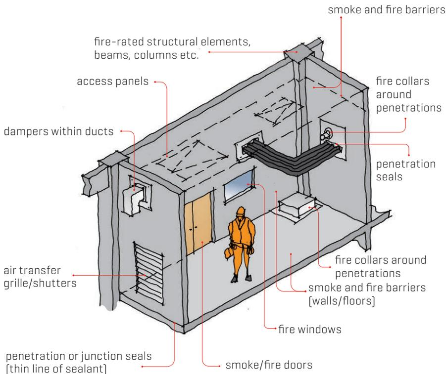
Figure 1. Passive fire protection building components
