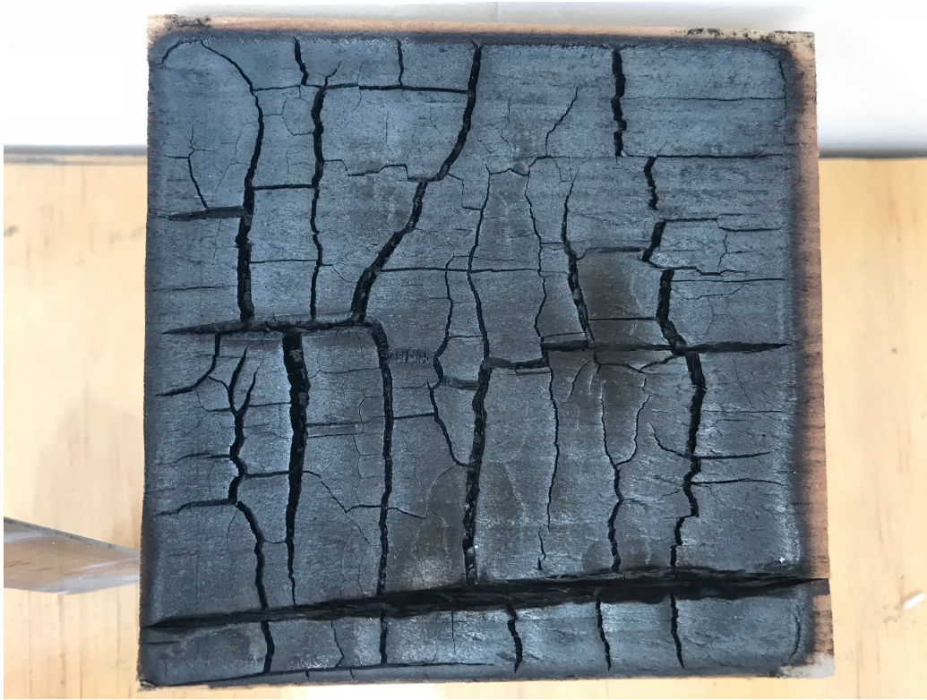
Figure 4. Photo of typical cracking that occurs in the charred surface of a laminated veneer lumber specimen subjected to radiant heat.
