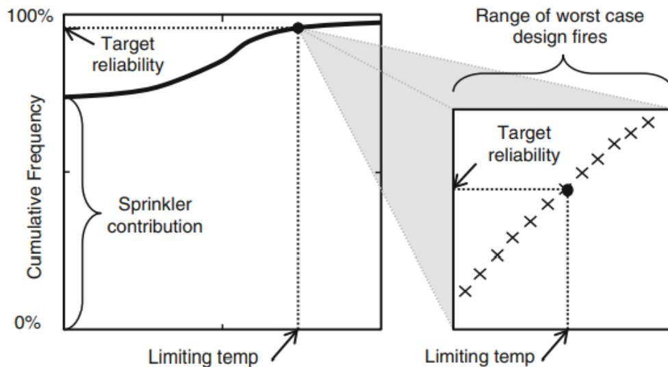
**Figure 34.** Determining the optimum fire resistance period [103]. Reprinted by permission from Springer.
