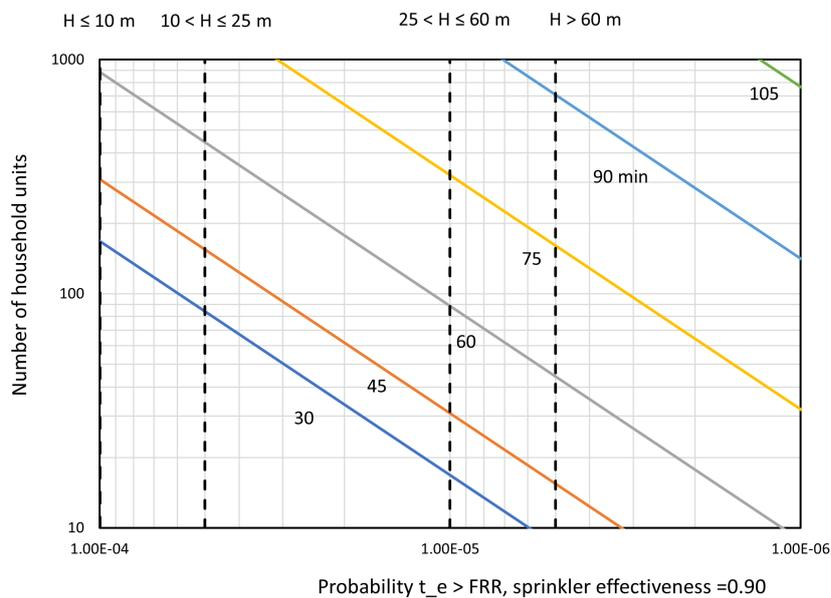
**Figure 50.** Failure probability curves for fire severities in the range 30 to 120 minutes, assuming the DIN EN 1991-1-2 NA + travelling fire model versus number of household units in the building with fire sprinklers of effectiveness 0.90. Vertical dashed lines indicate suggested target failure probabilities for buildings of various height, H.
