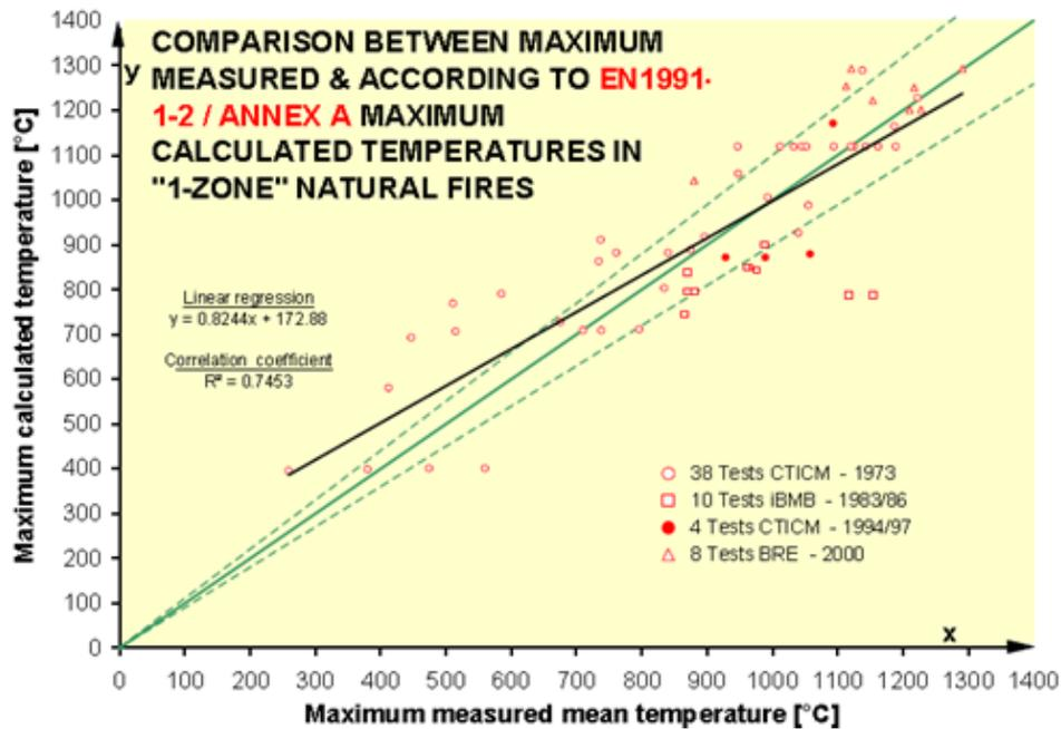
Figure 19. Parametric equations in EN1991-1-2:2002 compared to real fire tests [73].
