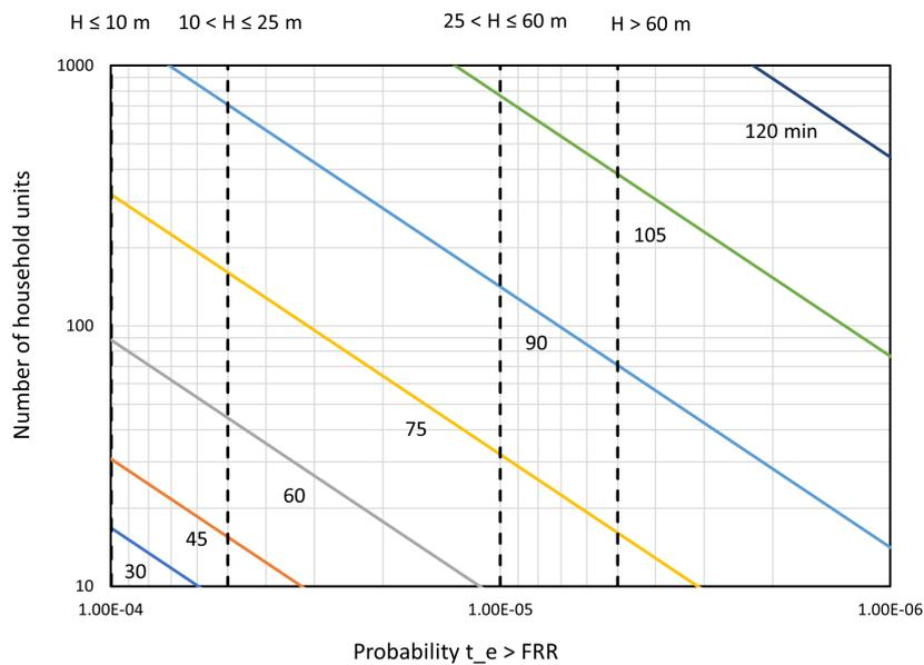
**Figure 49.** Failure probability curves for fire severities in the range 30 to 120 minutes, assuming the DIN EN 1991-1-2 NA + travelling fire model versus number of household units in the building without fire sprinklers. Vertical dashed lines indicate suggested target failure probabilities for buildings of various height, H.
