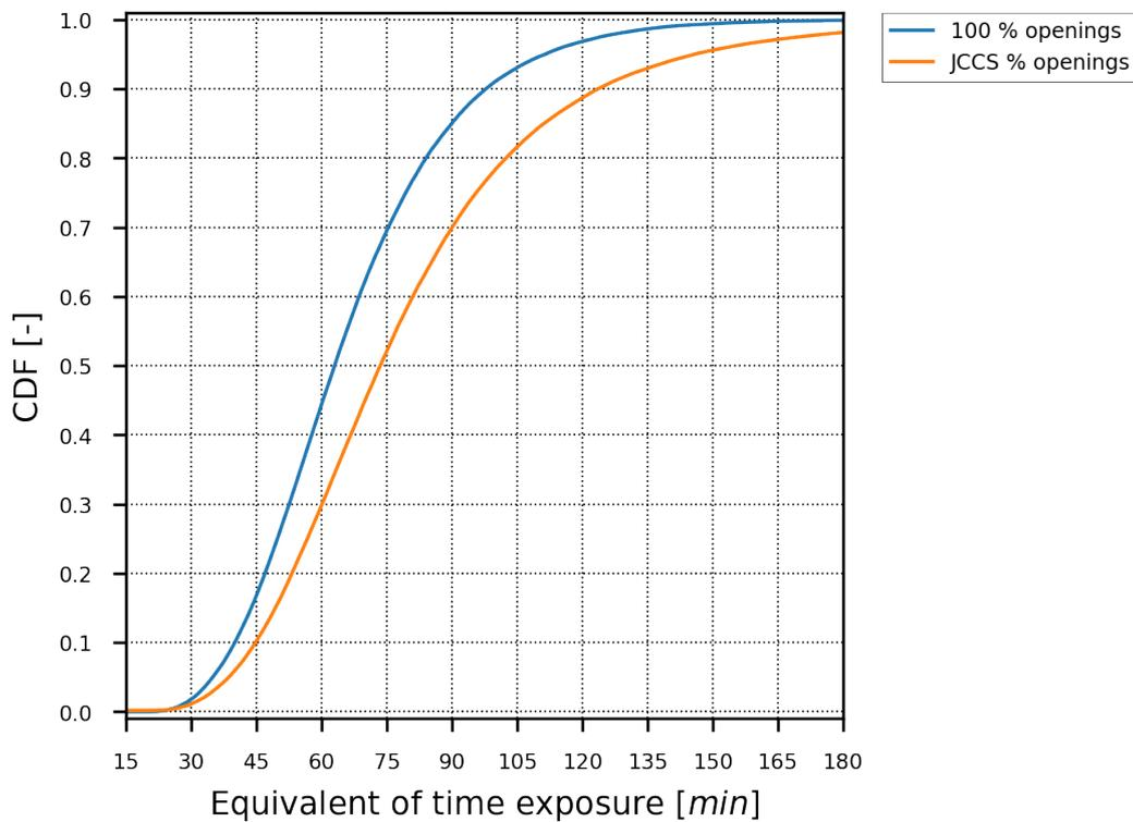
**Figure 41.** CDF comparing 100 % of window ventilation versus partial window breakage following JCCS truncated log-normal distribution with 100,000 simulations.
