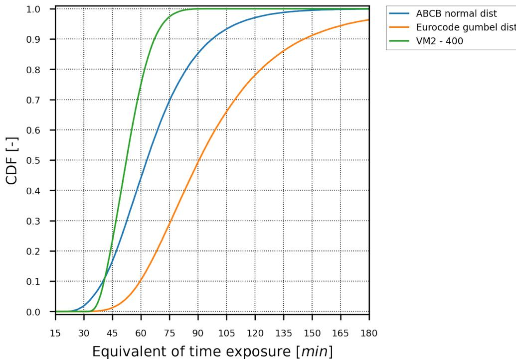
**Figure 42.** CDF comparing fire load assumptions for residential occupancies based on ABCB normal distribution, EN 1991-1-2 gumbel distribution and C/VM2 constant 400 MJ/m<sup>2</sup> with 100,000 simulations.
