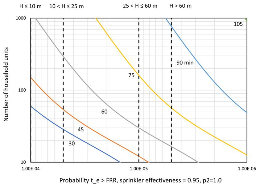
**Figure 54.** Failure probability curves for fire severities in the range 30 to 120 minutes, assuming the DIN EN 1991-1-2 NA + travelling fire model versus number of household units in the building with fire sprinklers of effectiveness 0.95 and ignoring fire service intervention  $p_2=1$ . Vertical dashed lines indicate suggested target failure probabilities for buildings of various height,  $H$ .
