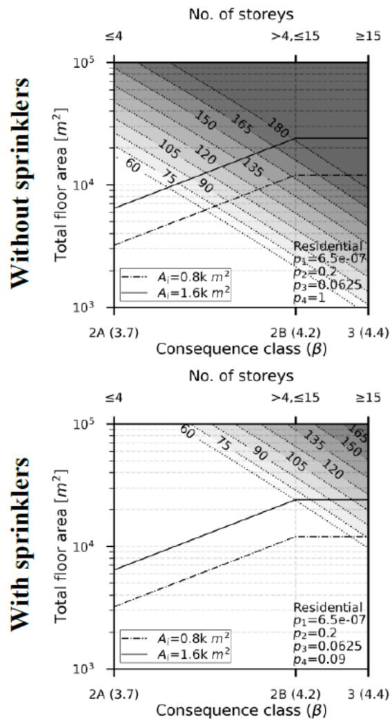
**Figure 38.** Contour plots of the solved structural fire-resistance rating at various building heights and total floor area (without and with sprinklers);  $A_i$  denotes floor area per storey. Extracted from [106].
