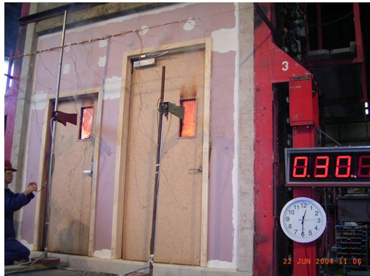
**Figure 4.** Fire doors during a standard fire resistance test. (Photo BRANZ Ltd).
