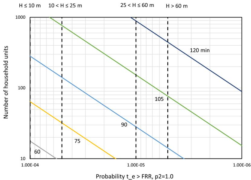
**Figure 52.** Failure probability curves for fire severities in the range 30 to 120 minutes, assuming the DIN EN 1991-1-2 NA + travelling fire model versus number of household units in the building without fire sprinklers and ignoring fire service intervention  $p_2=1$ . Vertical dashed lines indicate suggested target failure probabilities for buildings of various height, H.
