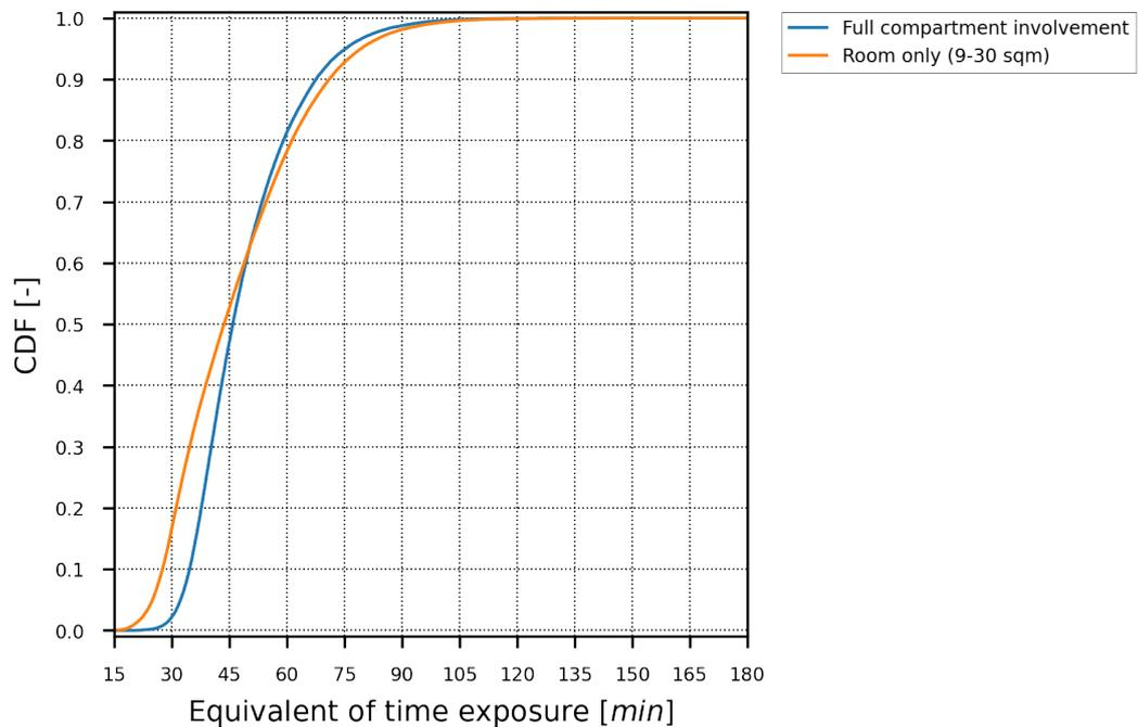
**Figure 43.** CDF comparing full compartment involvement based on Stats NZ data for size of household units versus room only involvement in the range 9 to 30 m<sup>2</sup> with 100,000 simulations.
