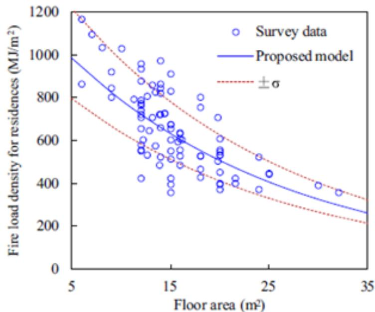
**Figure 16.** Comparison between fire load density model and survey data for residential buildings [51]. Reprinted by permission from Springer.
