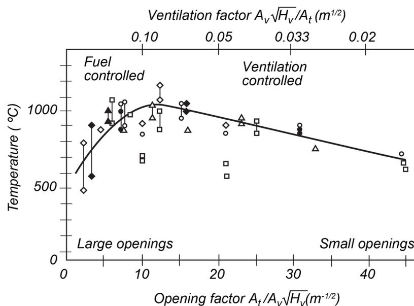
**Figure 15.** Maximum temperature measured inside the compartment vs the opening factor [29]. (Redrawn: Building Research Establishment.)
