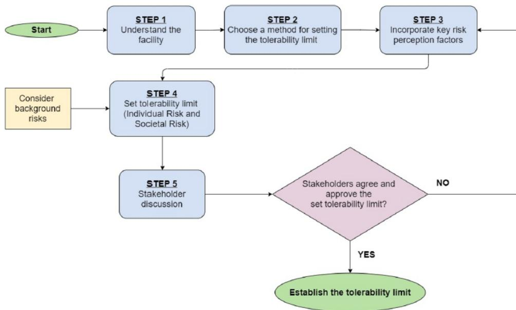
**Figure 28.** Proposed procedure for setting the tolerability limit for fire engineering PRA. [94]. Reprinted by permission from Springer.
