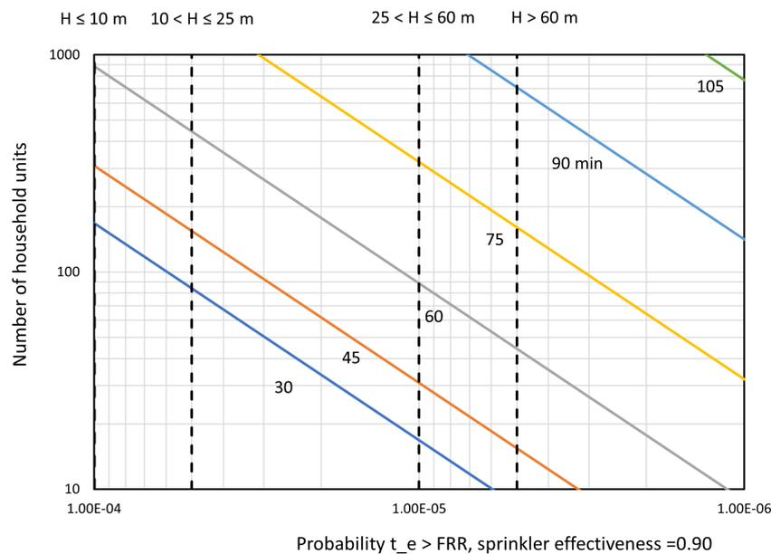
**Figure E2.** Failure probability curves for fire severities in the range 30 to 120 minutes, assuming the DIN EN 1991-1-2 NA + travelling fire model versus number of household units in the building with fire sprinklers of effectiveness 0.90. Vertical dashed lines indicate suggested target failure probabilities for buildings of various height, H.
