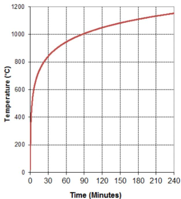
**Figure 5.** Standard time temperature curve [5].
