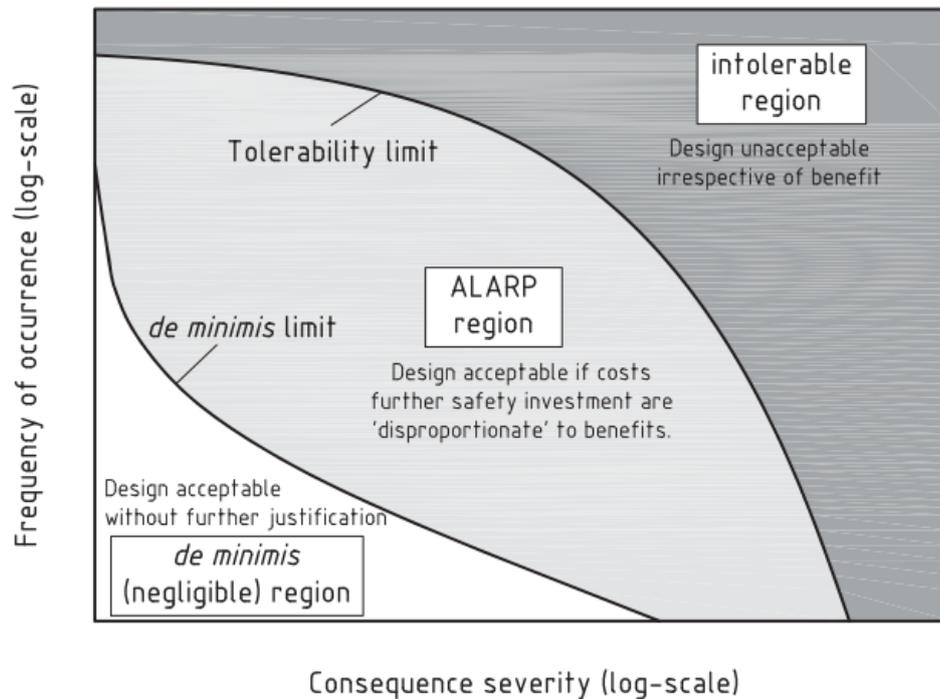
**Figure 27.** Illustrative fN curve – Societal acceptance criterion for a disaster: Relationship between consequence severity (event severity) and the frequency of event (event likelihood). Extracted from [83]. Reprinted by permission from Springer.
