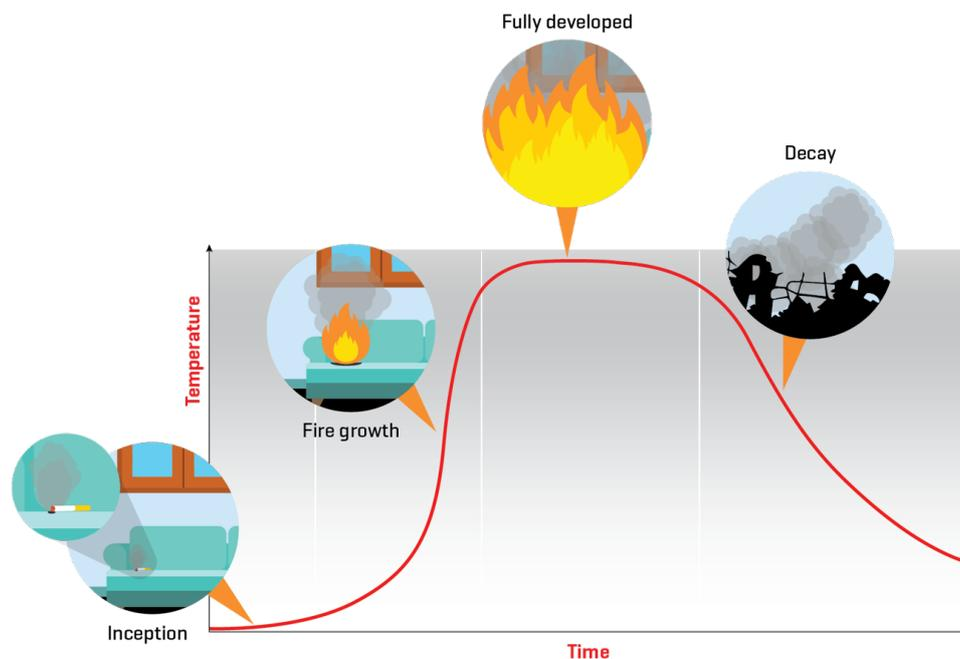
**Figure 3.** Time temperature and different stages describing the course of a fire. (Image BRANZ Ltd.)
