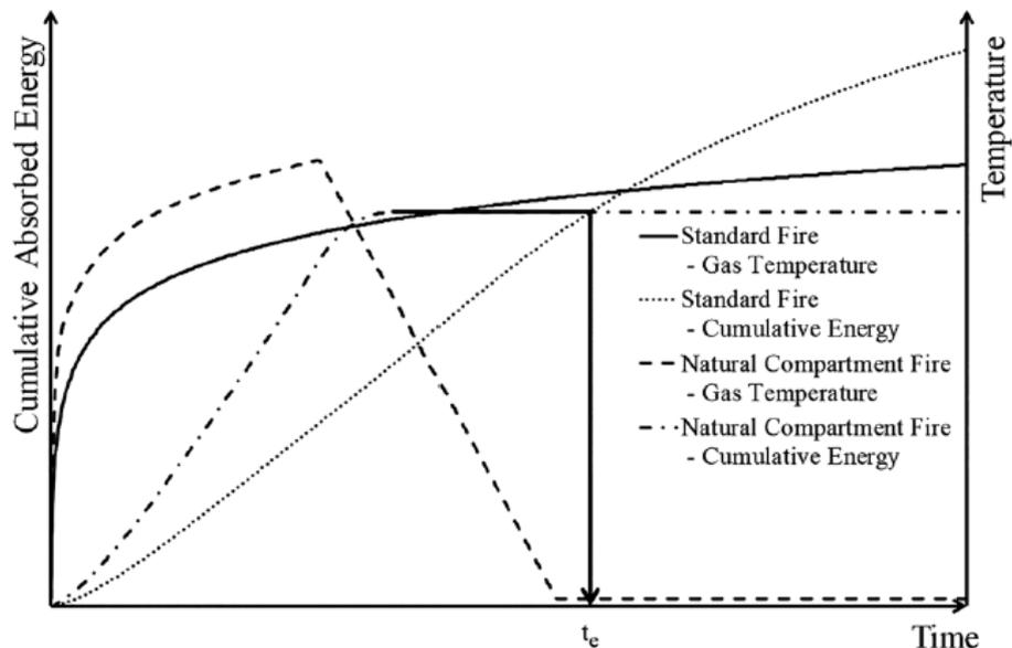
**Figure 7.** A graphical representation of the equal energy time equivalence calculation. Reproduced from MacIntyre et al. [9].
