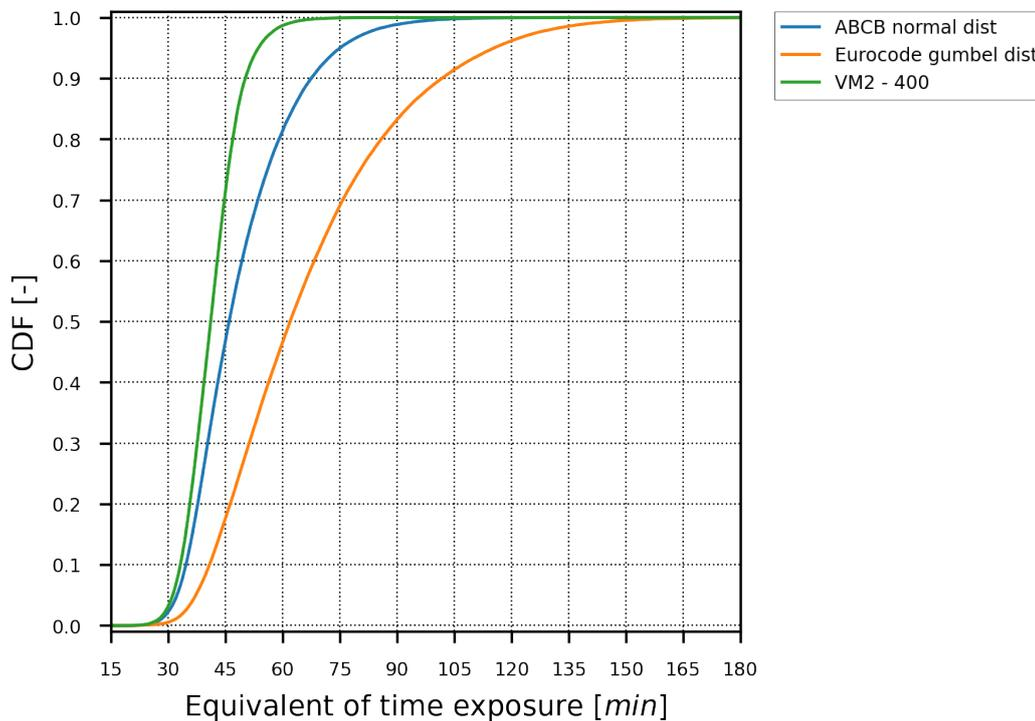
**Figure 45.** CDF comparing fire load assumptions for residential occupancies based on ABCB normal distribution, EN 1991-1-2 gumbel distribution and C/VM2 constant 400 MJ/m<sup>2</sup> with 100,000 simulations.
