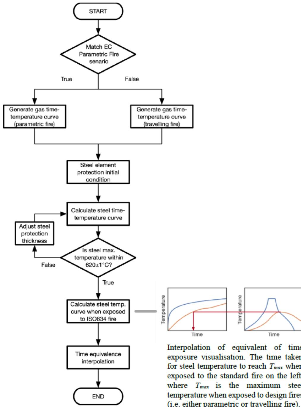
**Figure 36.** The process of a single MCS in determining structural fire resistance. Extracted from [74].
