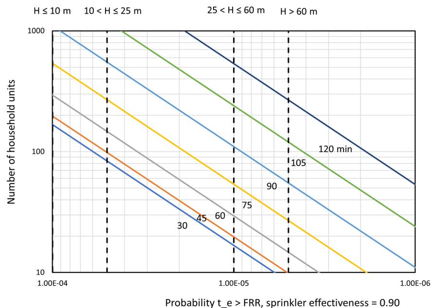
**Figure 47.** Failure probability curves for fire severities in the range 30 to 120 minutes, assuming the EN 1991-1-2 Annex A fire model versus number of household units in the building with fire sprinklers of assumed effectiveness 0.90. Vertical dashed lines indicate suggested target failure probabilities for buildings of various height, H.
