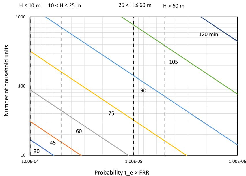
**Figure E1.** Failure probability curves for fire severities in the range 30 to 120 minutes, assuming the DIN EN 1991-1-2 NA + travelling fire model versus number of household units in the building without fire sprinklers. Vertical dashed lines indicate suggested target failure probabilities for buildings of various height, H.
