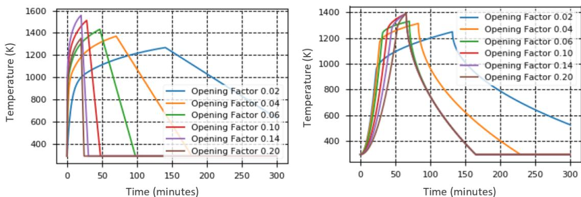
Figure 20. Parametric time temperature curves EN 1991-1-2 Annex A (left) and DIN EN 1991-1-2/NA (right). Adapted from [74].
