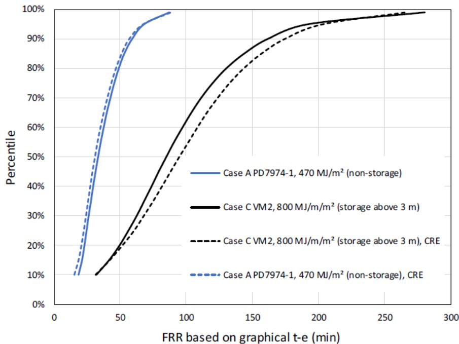
**Figure 35.** Comparing cumulative frequency distribution for FRR based on t-e and FRR based on CRE method. Extracted from Wade and Frank [105].
