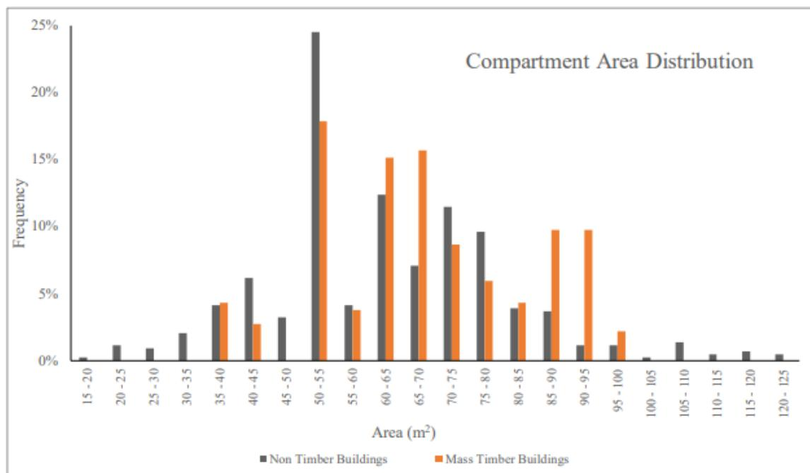
**Figure 13.** Compartment area frequencies from residential buildings (n=513 for non-timber buildings and n=185 for mass timber buildings) [27]. (Image: RISE, Sweden.)
