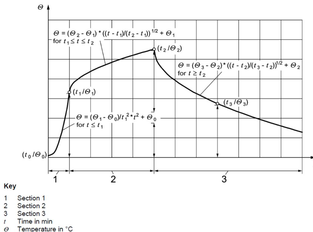
**Figure 21.** Mathematical description of the DIN EN 1991-1-2/NA:2010-12 parametric time temperature curves parametric fire curves in 3 sections. Extracted from [61].
