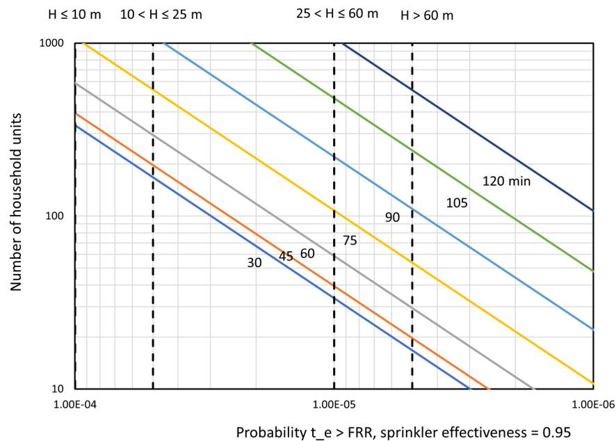
**Figure 48.** Failure probability curves for fire severities in the range 30 to 120 minutes, assuming the EN 1991-1-2 Annex A fire model versus number of household units in the building with fire sprinklers of assumed effectiveness 0.95. Vertical dashed lines indicate suggested target failure probabilities for buildings of various height, H.
