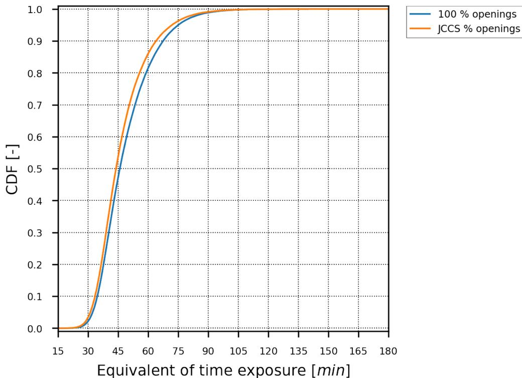
**Figure 44.** CDF comparing 100 % of window ventilation versus partial window breakage following JCCS truncated log-normal distribution with 100,000 simulations.
