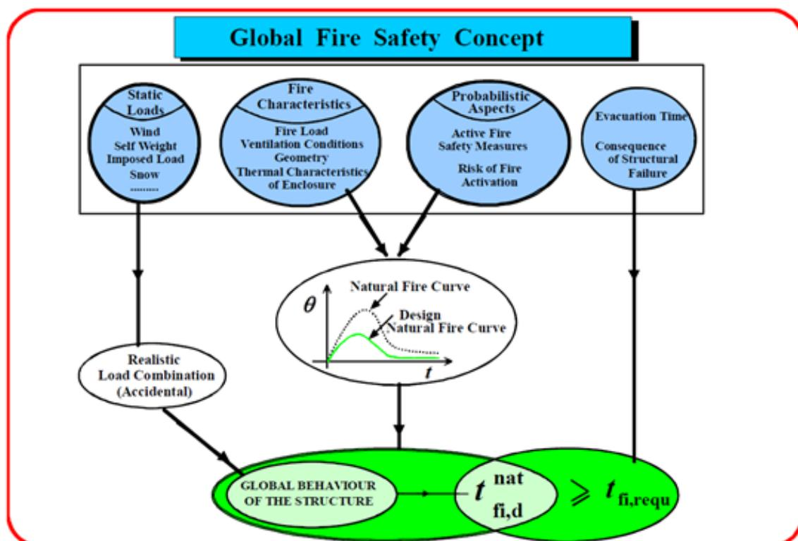
**Figure 23.** Successive steps of the global fire safety concept. Extracted from Schleich [73].
