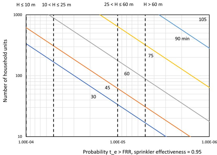
**Figure 51.** Failure probability curves for fire severities in the range 30 to 120 minutes, assuming the DIN EN 1991-1-2 NA + travelling fire model versus number of household units in the building with fire sprinklers of effectiveness 0.95. Vertical dashed lines indicate suggested target failure probabilities for buildings of various height, H.
