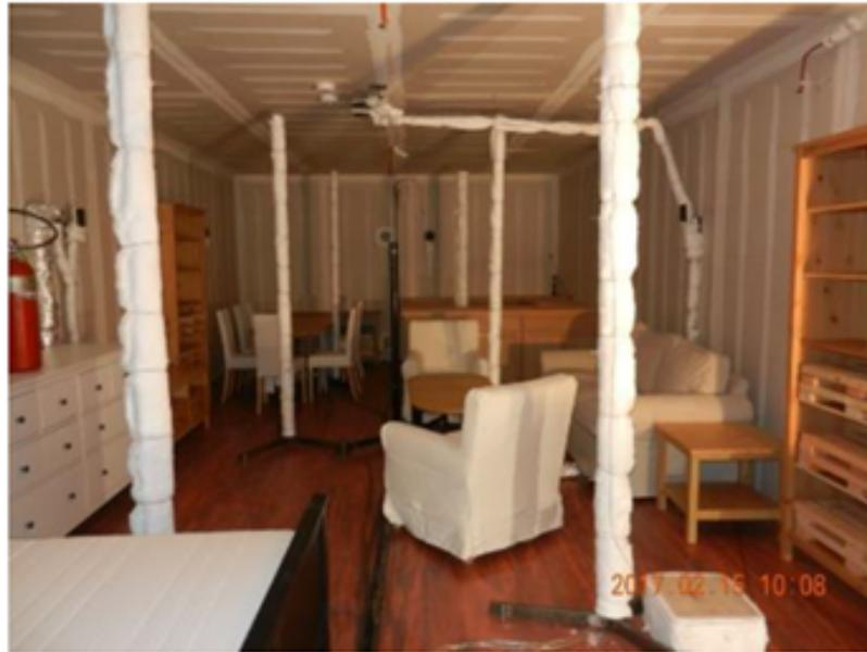
**Figure 17.** Photo of the moveable fire load used in full scale fire testing where the fire load energy density was 550 MJ/m<sup>2</sup> [53]. Reprinted by permission from National Research Council.
