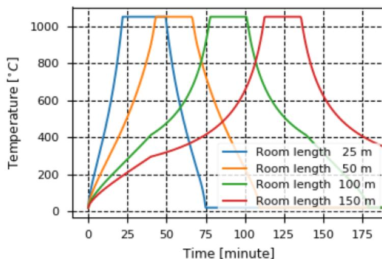
**Figure 22.** Example travelling time-temperature at structural element. Extracted from from [74].
