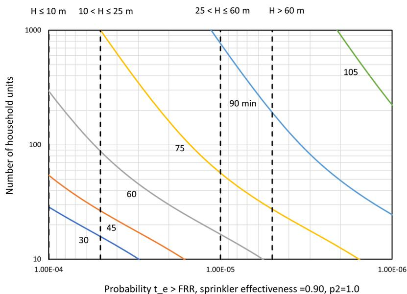
**Figure 53.** Failure probability curves for fire severities in the range 30 to 120 minutes, assuming the DIN EN 1991-1-2 NA + travelling fire model versus number of household units in the building with fire sprinklers of effectiveness 0.90 and ignoring fire service intervention  $p_2=1$ . Vertical dashed lines indicate suggested target failure probabilities for buildings of various height, H.
