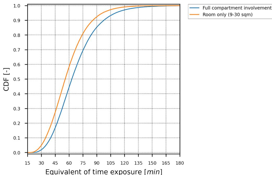
**Figure 40.** CDF comparing full compartment involvement based on Stats NZ data for size of household units versus room only involvement in the range 9 to 30 m<sup>2</sup> with 100,000 simulations.
