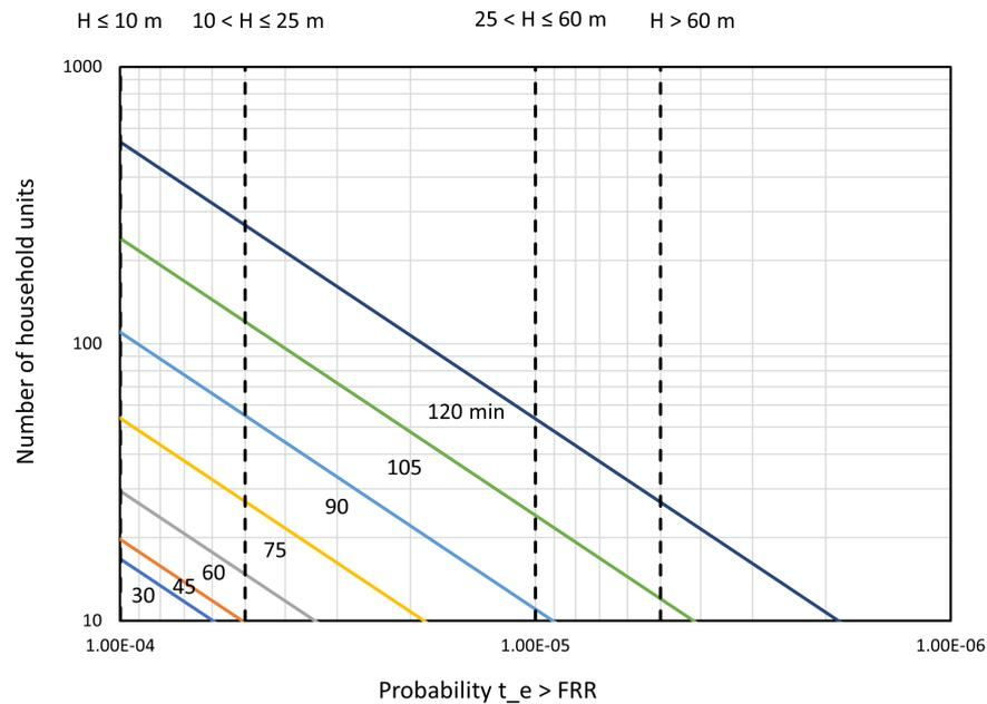
**Figure 46.** Failure probability curves for fire severities in the range 30 to 120 minutes, assuming the EN 1991-1-2 Annex A fire model versus number of household units in the building without fire sprinklers. Vertical dashed lines indicate suggested target failure probabilities for buildings of various height, H.
