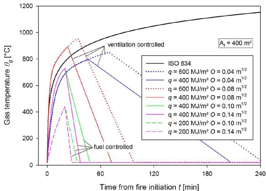
**Figure 18.** ISO 834 standard fire and EN 1991-1-2 parametric fires for different fire load and ventilation [72].
