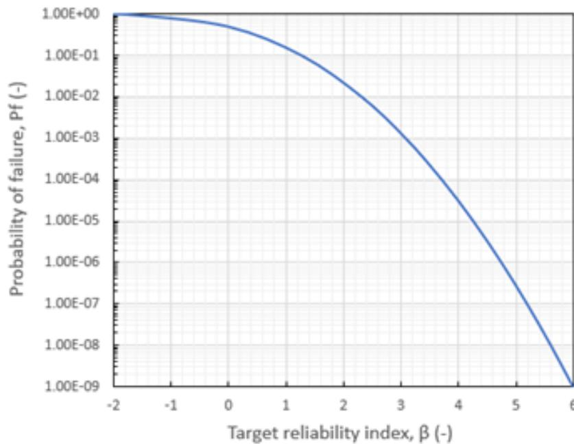
**Figure 24.** Relationship between probability of failure and the target reliability index.
