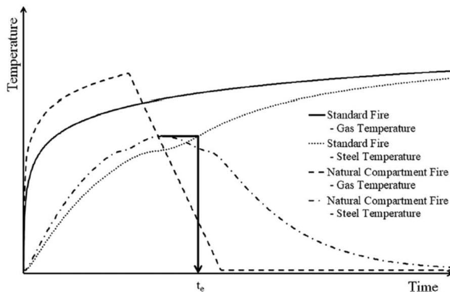
**Figure 6.** A graphical representation of the maximum temperature time-equivalence calculation. Reproduced from MacIntyre et al. [9].
