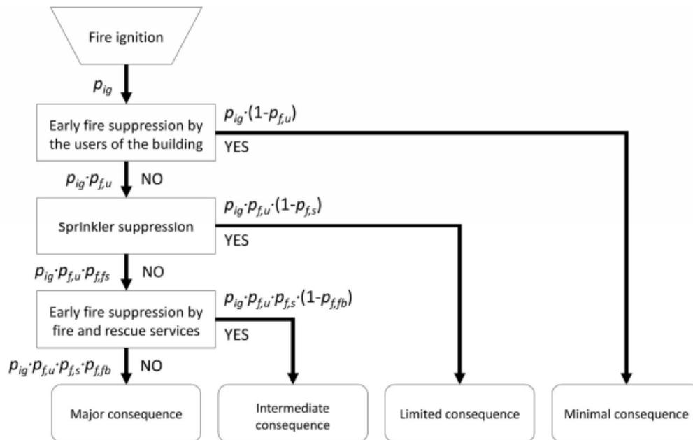
**Figure 26.** Concept probability tree – The consequence of fire occurrence are dependent on sprinkler operation. Extracted from [83].
