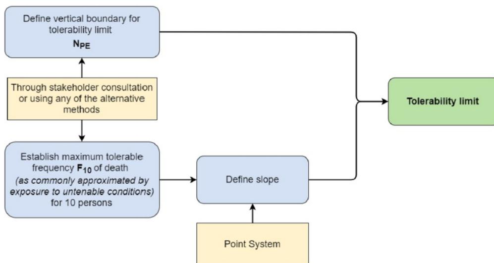
**Figure 29.** Flowchart illustrating the steps for setting up a societal tolerability limit. [94]. Reprinted by permission from Springer.
