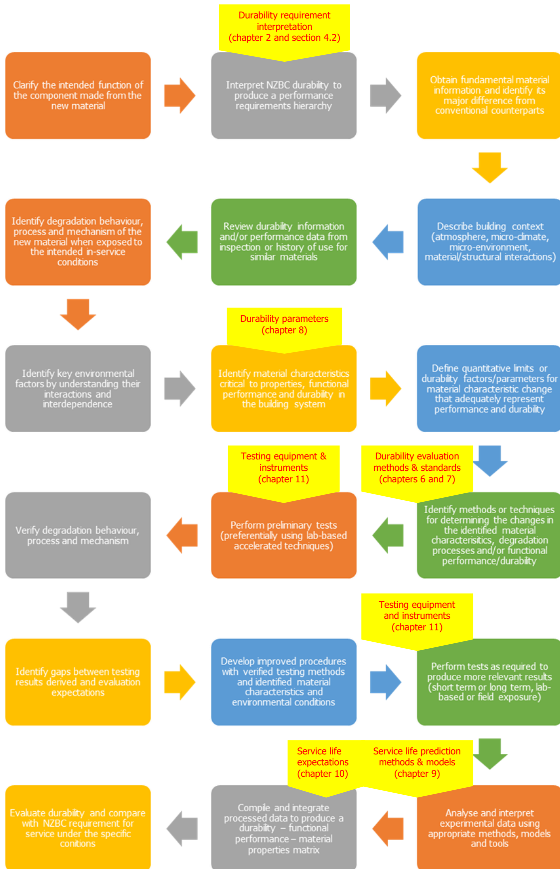
Figure 5. A general approach to develop schemes for durability evaluation of new materials.
