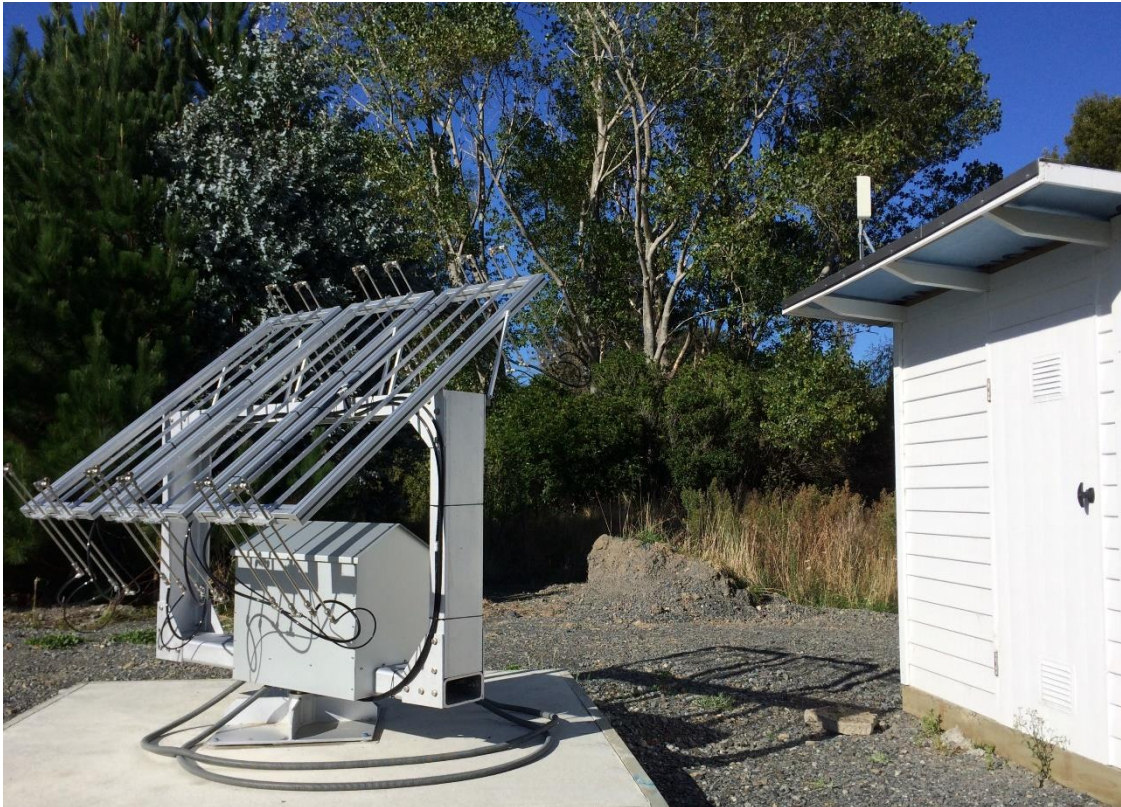
Figure 25. The weathering rig developed in this study.
