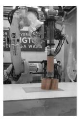
Robot 3D printing computationally generated clay column with ornamentation
