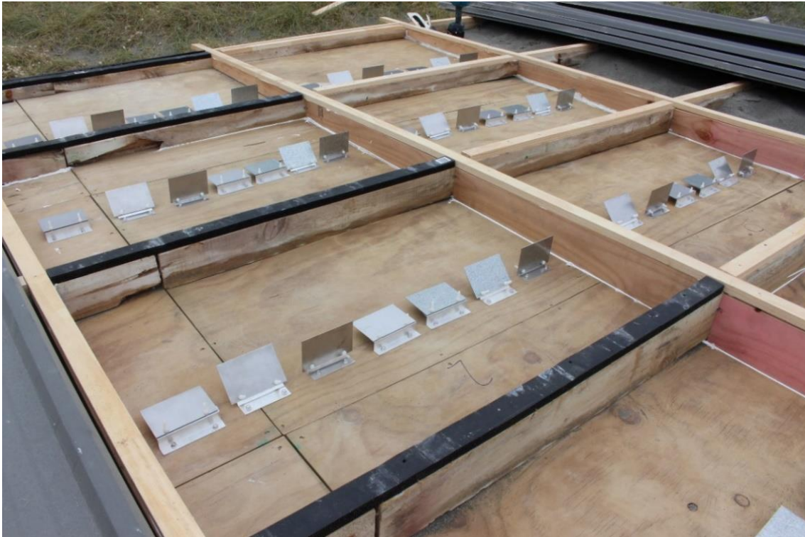
Figure 2. Vented and unvented roof cavity of the test structure with metal coupons already in place.
