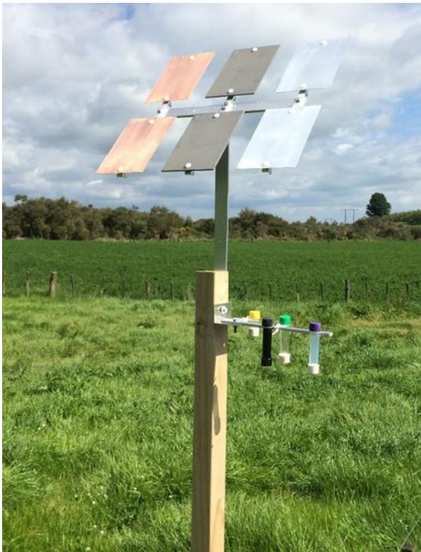
Figure 4. A typical exposure rack with a selection of passive tube sensors.
