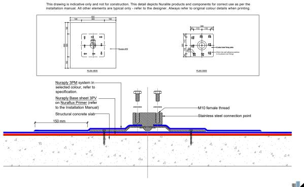
SECTIONAL ELEVATION: CENTRE FIXING NOT SHOWN
