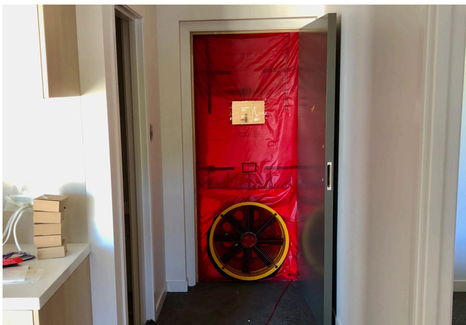
Blower door fan mounted in entrance doorway.
