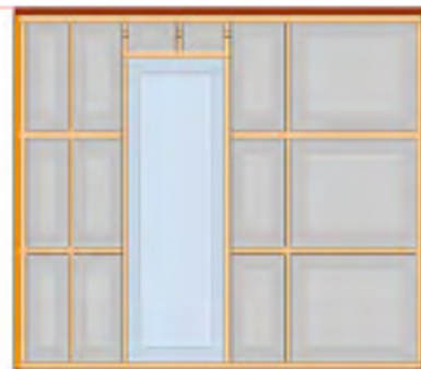
Construction R-value with R2.0 insulation, R1.79 Construction R-value with R2.8 insulation, R2.00 Framing ratio 23%
