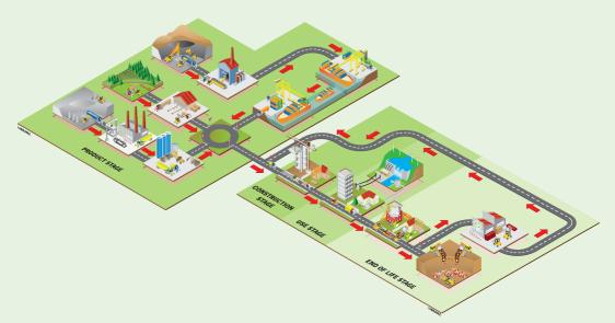
Building LCA is a tool for quantifying the potential environmental impacts of a building through its use of resources and energy across the life cycle. The assessment is systematic and requires making an inventory of the activities that are collectively needed to produce, operate and ultimately dispose of the building being investigated.
