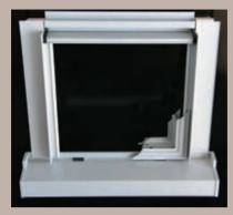
The Flashman Flashing System is New Zealand designed, manufactured and factory fabricated, then fitted on site by Approved Installers. This complete low maintenance flashing system expels moisture from the head and sides of windows via the extruded aluminium sill. The sill supports the bottom of the window or door and double glazing. The aluminium sill is 1.8 mm thick and powder coated. The system allows cladding to be fitted with or without facings. For more information see www.flashman.co.nz.
