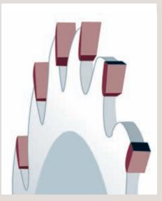
**Flat-top grind (FTB):** has straight chisel teeth for ripping i.e. cutting parallel to the wood fibres. It cuts a kerf with a smooth square bottom, but will splinter the grain if used to cross-cut.
