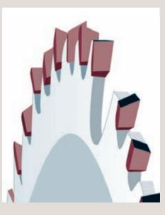
Alternate top bevel with raker (ABT & R): has a chisel-shaped raker tooth after every two pairs of alternating top-bevel ground teeth to clean up the kerf. A good all-rounder when you want one blade to rip and cross-cut.
