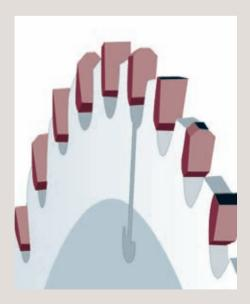
**Triple-chip grind (TCG):** has teeth which are alternately flat tops and ones chamfered on each edge. The chamfered tooth cuts out the middle of the kerf, then the flat-top follows and cleans out the corners. A good design for particleboard, laminates and hardwoods.
