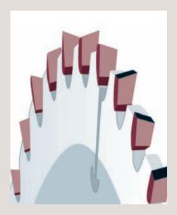
Alternate top bevel (sometimes given as ATB on the blade packaging): has every tooth ground at an angle in alternate directions. The teeth cut the grain rather than tearing it, making it a good choice for cross-cutting.
