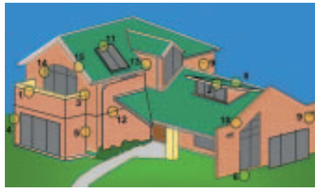
Figure 1. Flashings must be an integral part of the design and construction of the cladding
