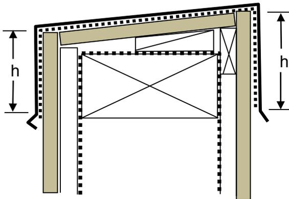
Barge flashing for profiled metal
