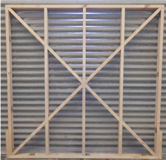
Figure 28. Specimen for double diagonal braces cut between studs
