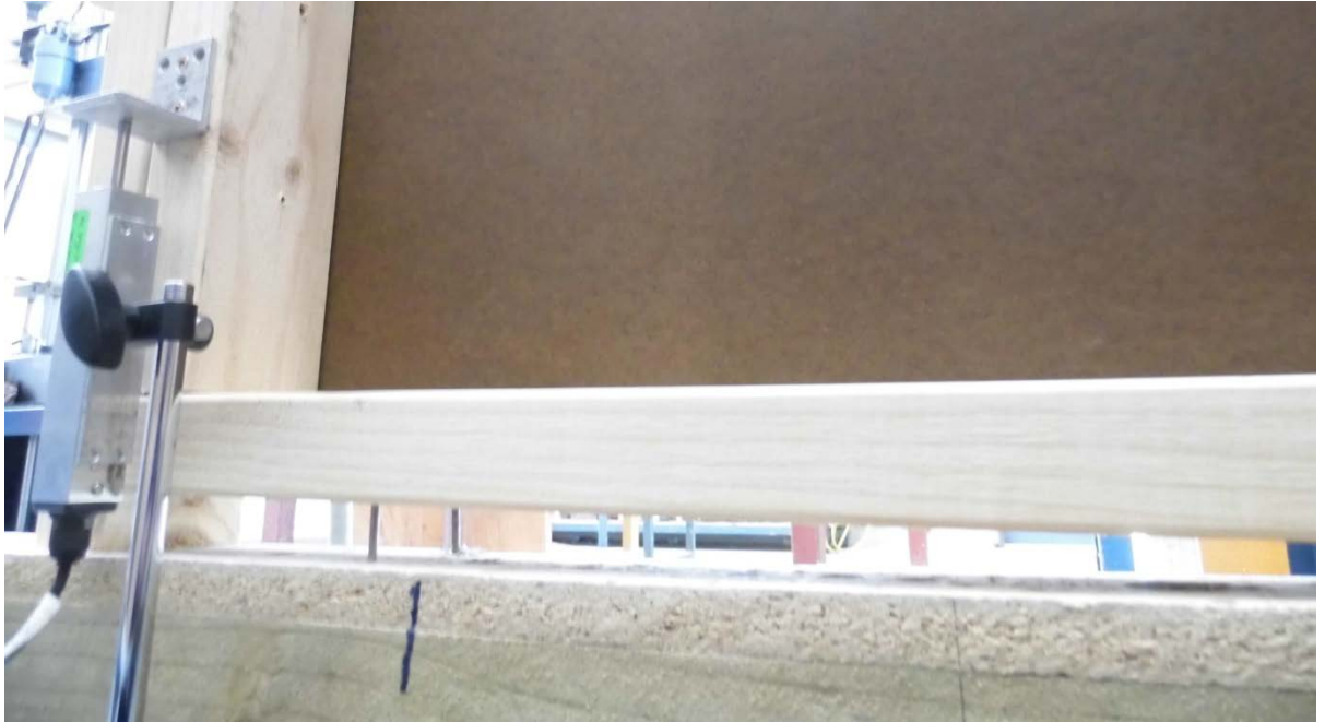
Figure 56. Sheet 3 bottom plate lifting in hardboard-lined specimen fixed with clouts and no extra hold-down
