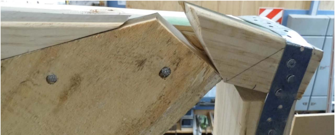
Figure 18. Diagonal brace lifts top plate in tests after connection strengthening
