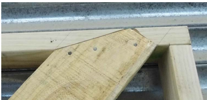
Figure 14. Joint at top plates in specimen for 150 x 25 let in brace at 45°
