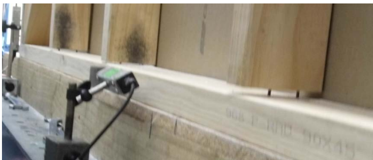
Figure 74. Middle studs lifting in Combo 1
