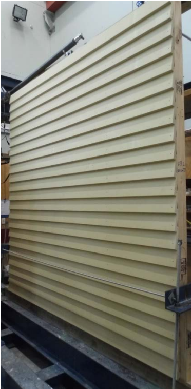
Figure 45. Specimen for weatherboard wall Board 2
