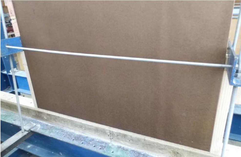
Figure 52. Sheet 3 hardboard single-lined specimen fixed with panel pins
