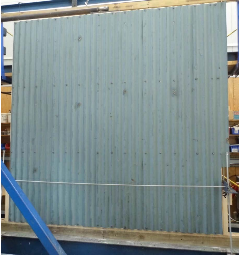
Figure 64. Front view of Sheet 5 – vertical corrugated steel
