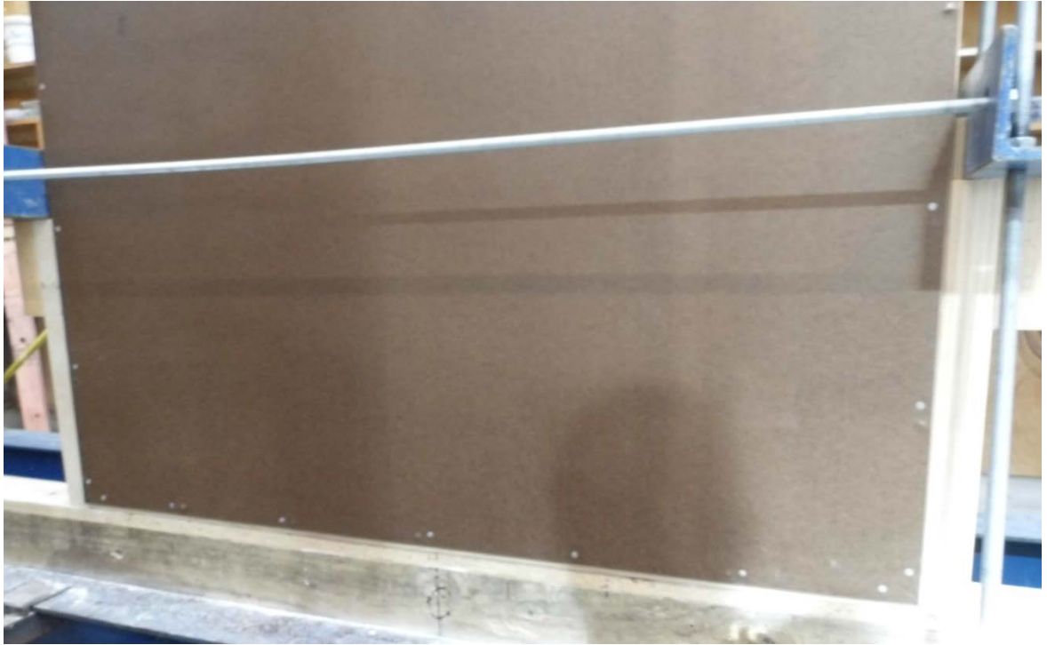
Figure 54. Sheet 3 hardboard single-lined specimen fixed with clouts
