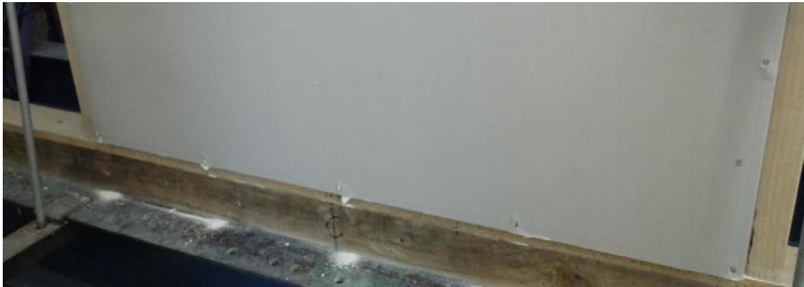
Figure 50. Sheet 2 standard plasterboard lined on both sides of specimen
