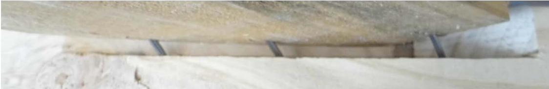
Figure 18. Diagonal brace lifts top plate in tests after connection strengthening
