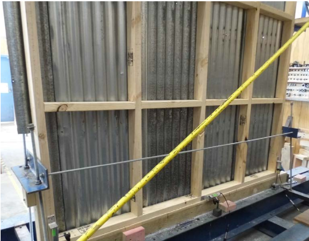
Figure 65. Back view of Sheet 5 – vertical corrugated steel
