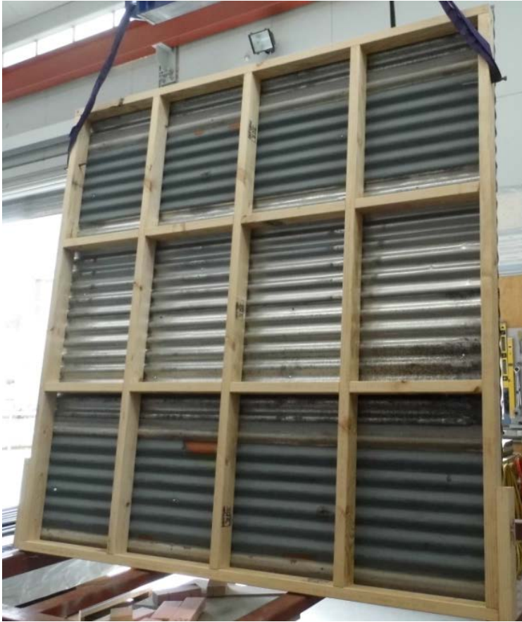
Figure 59. Back view of Sheet 4 – horizontal corrugated steel
