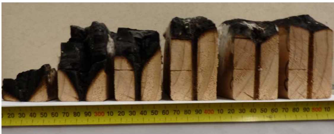
Figure 29: Cone-shaped charring progression in 6 mm holes, left to right, reducing furnace pressure from 11 Pa to -11 Pa (top to bottom) in BRANZ tests
