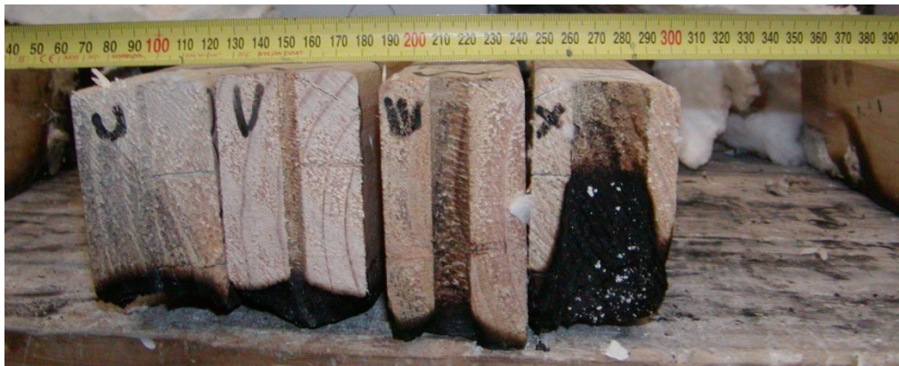
Figure 119: Charring in 3 to 24 mm holes at -11.96 Pa after 120 minutes (left to right U, V, W and X)
