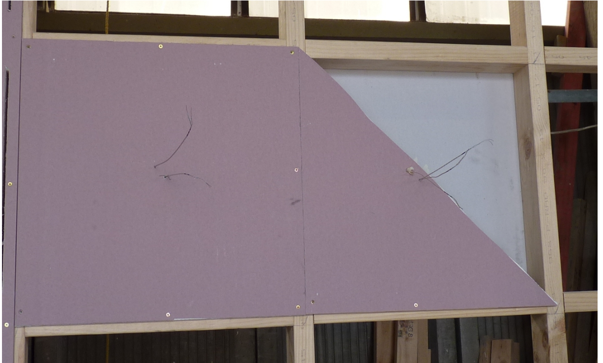
Figure 94: Left to right intact non-exposed lining and 1.5 mm crack in non-exposed lining
