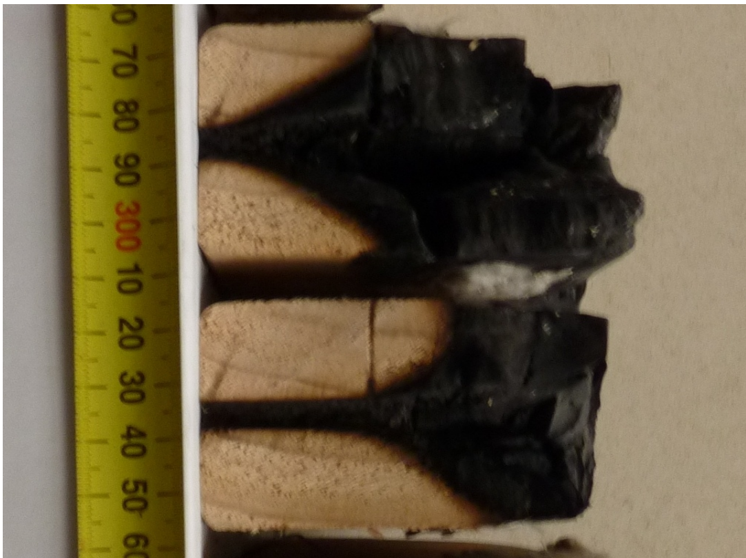
Figure 47: Cone-shaped charring profile in opposed-flame spread
