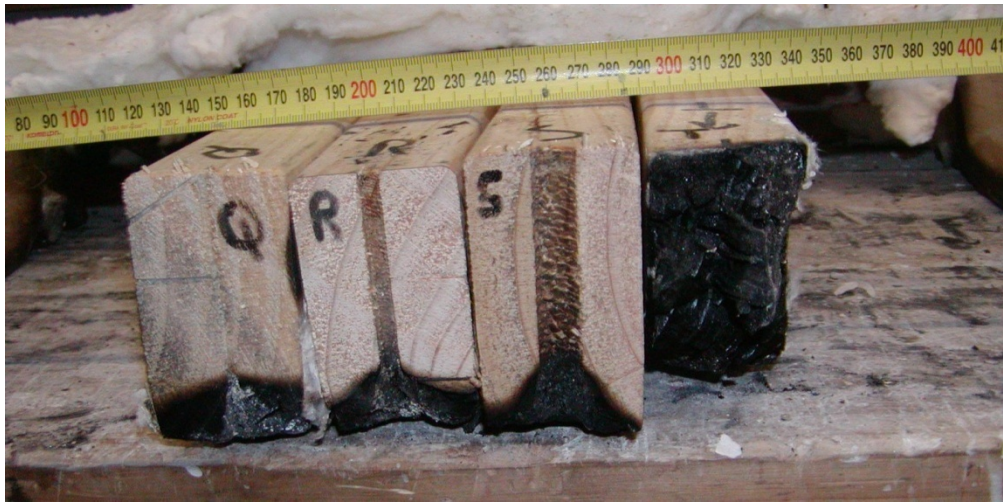
Figure 118: Charring in 3 to 24 mm holes at -7.24 Pa after 120 minutes (left to right Q, R, S and T)
