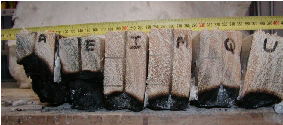
Figure 112: Charring in 3 mm holes after 120 minutes (left to right A, E, I, M, Q and U)
