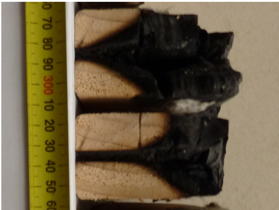
Figure 60: Extent of charring in 6 mm holes at 6.9 and 2.2 Pa furnace pressures
