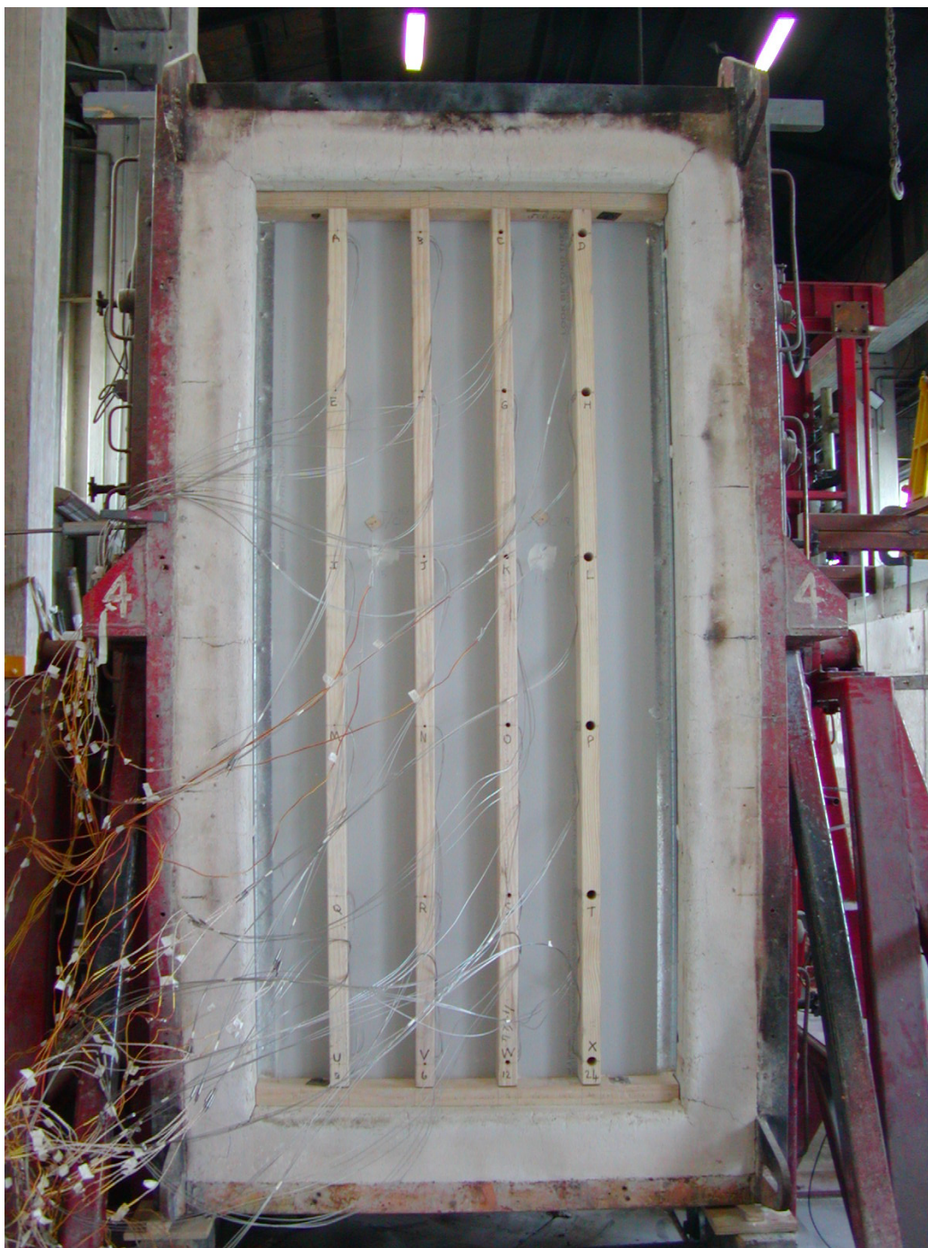
Figure 49: Test 1 pilot scale 3, 6, 12 and 24 mm holes at different elevations and furnace pressures
