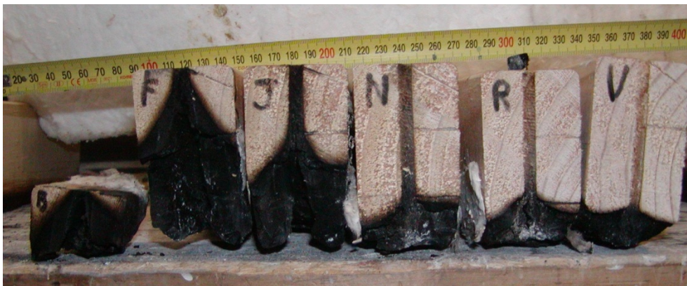
Figure 113: Charring in 6 mm holes after 120 minutes (left to right holes B, F, J, N, R and V)
