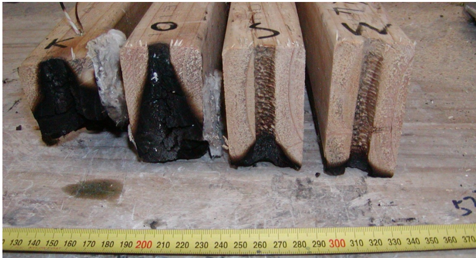
Figure 114: Charring in 12 mm holes after 120 minutes (left to right holes K, O, S and W)
