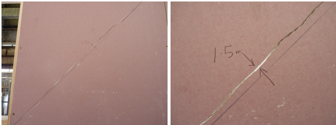
Figure 95: 1.5 mm crack on exposed side
