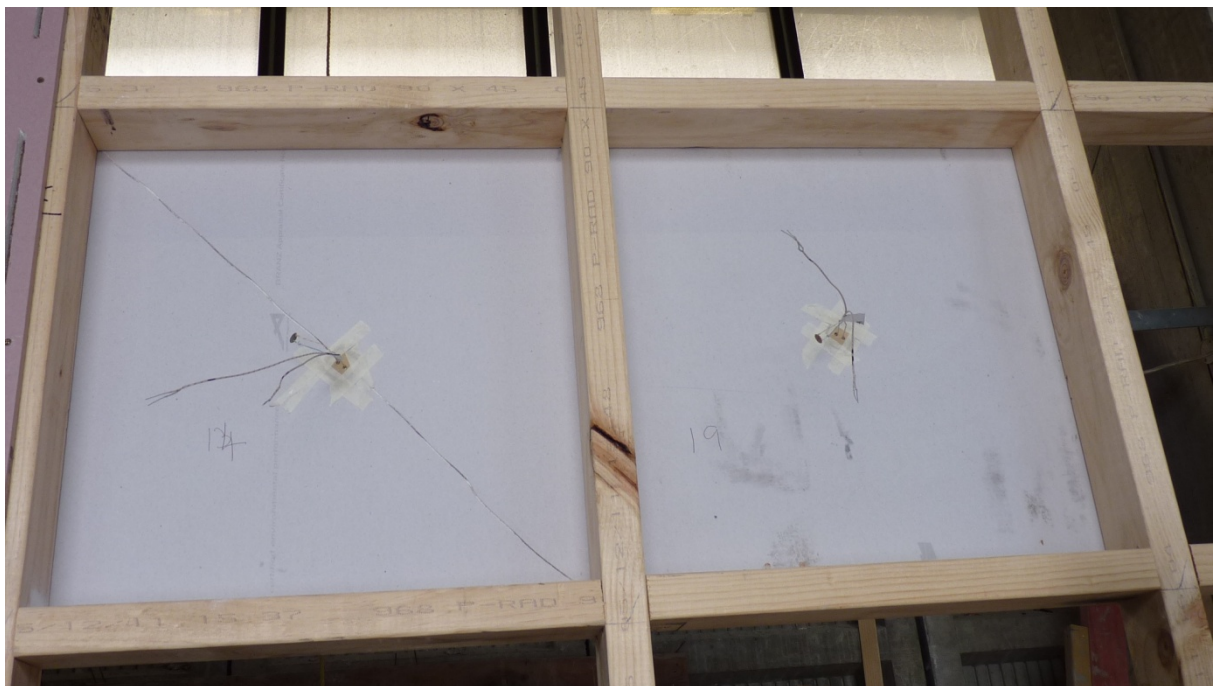
Figure 93: Left to right 1.5 mm crack on exposed lining and intact exposed lining
