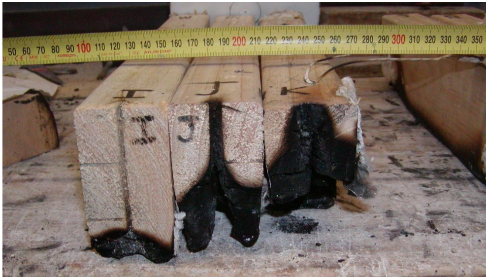
Figure 116: Charring in 3 to 12 mm holes at 2.2 Pa after 120 minutes (left to right I, J and K)
