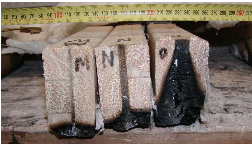
Figure 117: Charring in 3 to 12 mm holes at -2.52 Pa after 120 minutes (left to right M, N and O)
