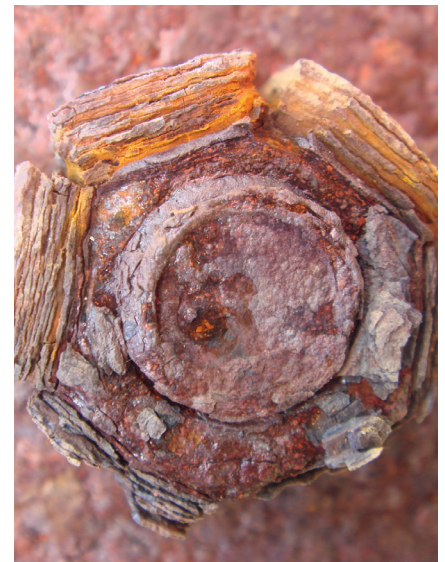
Figure 1. Mild steel nuts after 3 years' exposure to a rural atmosphere (left) and a severe marine atmosphere (right).
