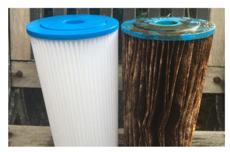
A new 20 micron water filter (left) and the used filter it is replacing after 4 months' use.
