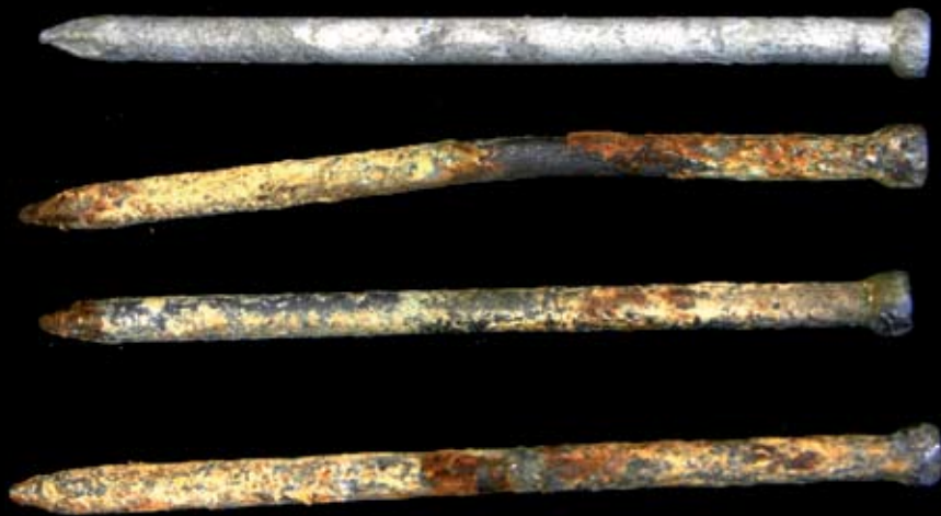
Nails taken from a non-sea spray zone deck in service for 7 years compared against a new one. The timber treatment here was also ACQ, but there was less moisture present in the treated timber.
