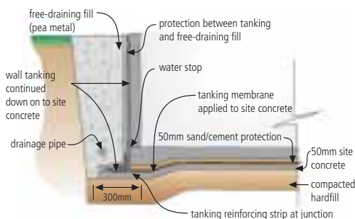
Figure 1: Section through typical tanked concrete wall
