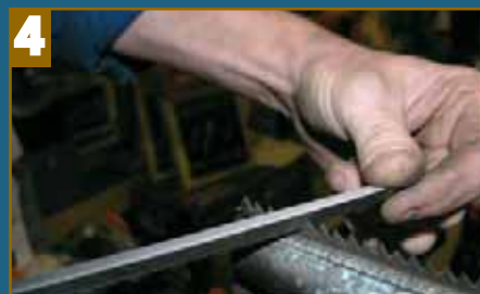
Arrange the saw so it is held about 3 mm above your clamp so it won't vibrate and screech as you file.
