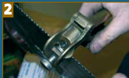
A setting tool has an anvil and a punch.
