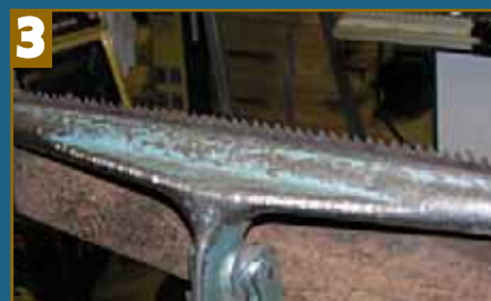
Arrange the saw so it is held about 3 mm above your clamp so it won't vibrate and screech as you file.
