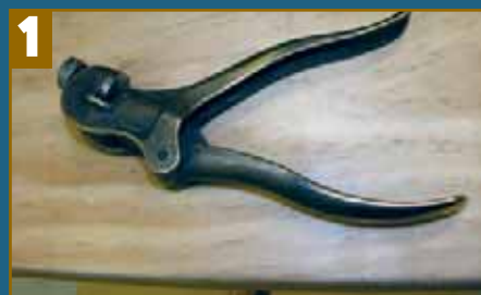
A setting tool has an anvil and a punch.
