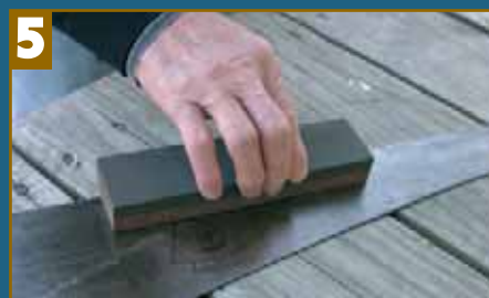
Rub a fine oilstone along each face of the saw to remove any burrs from filing.
