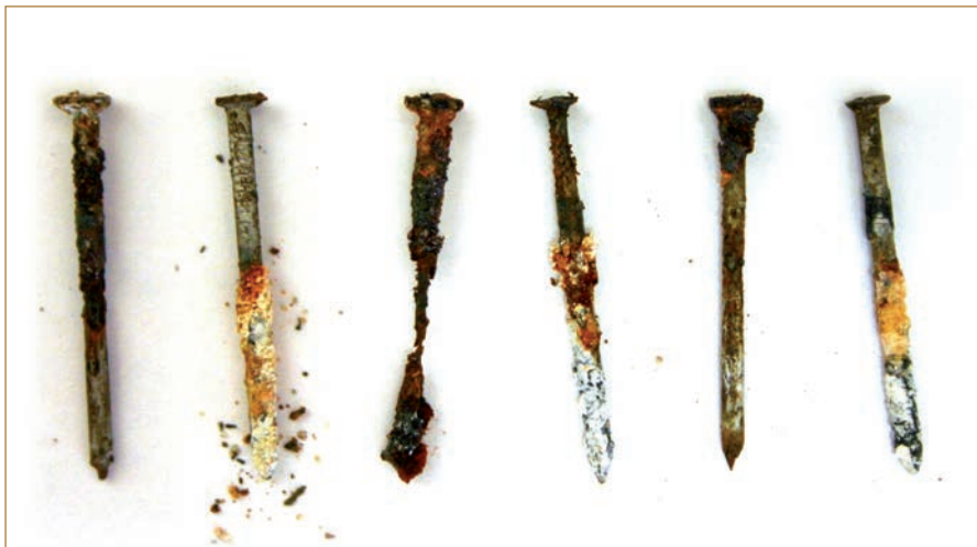
Galvanised steel nails after just 12 months in a high-humidity test in ACQ-treated timber. The decay shows the need for careful selection of fixings for each situation.
