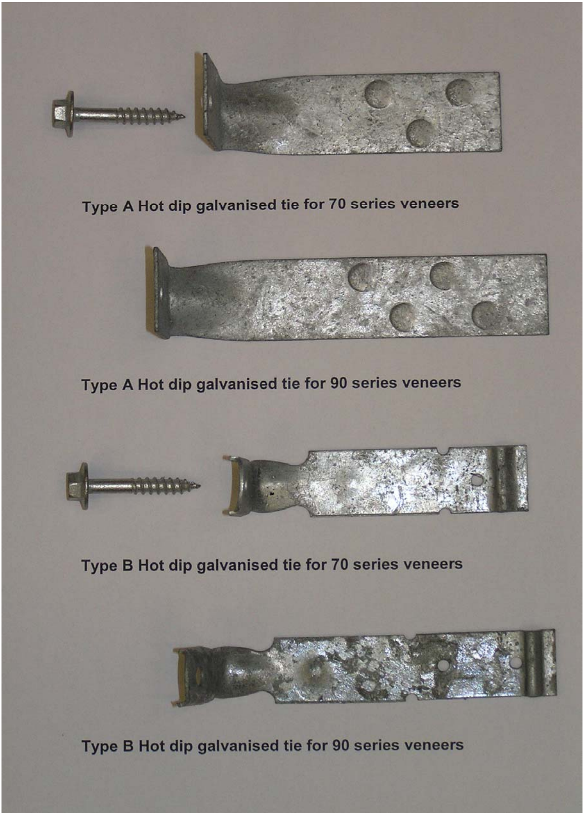
Figure 7: Hot-dipped galvanised ties
