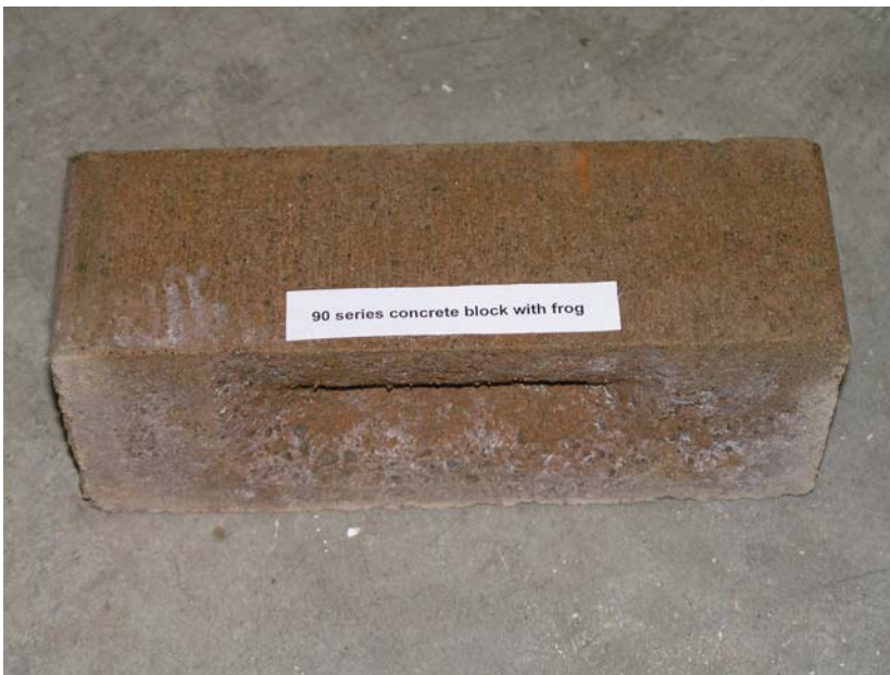
Figure 5: 90 series concrete block with "frog"
