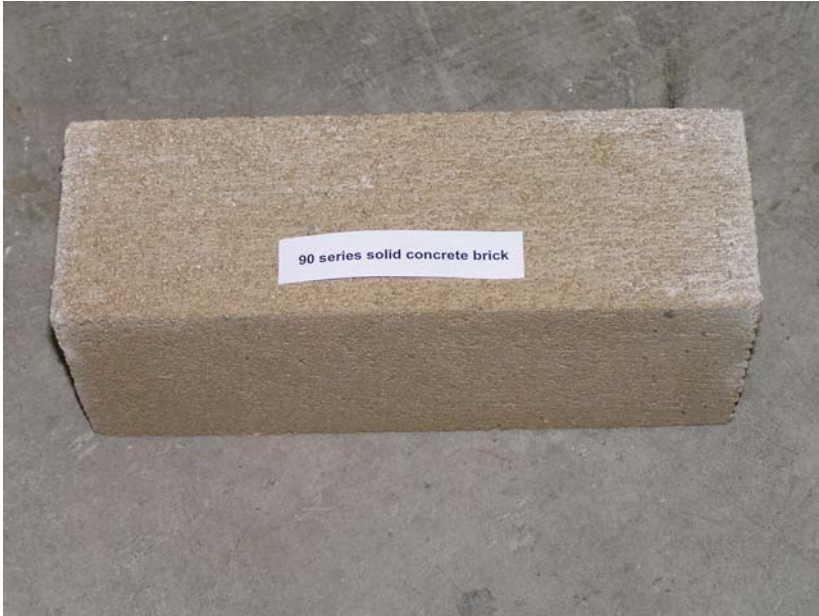
Figure 4: 90 series solid concrete block
