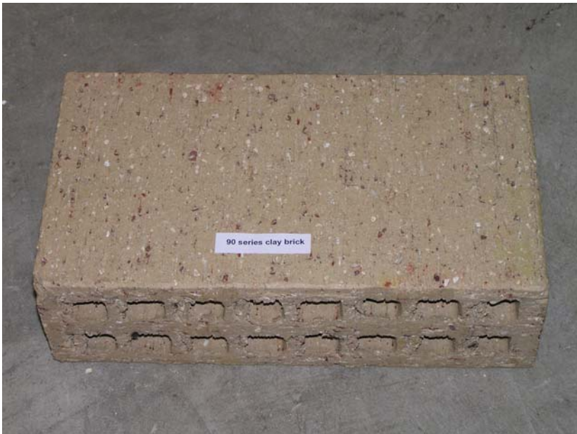
Figure 3: 90 series clay brick with holes
