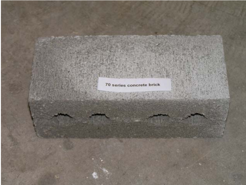
Figure 2: 70 series concrete block with holes
