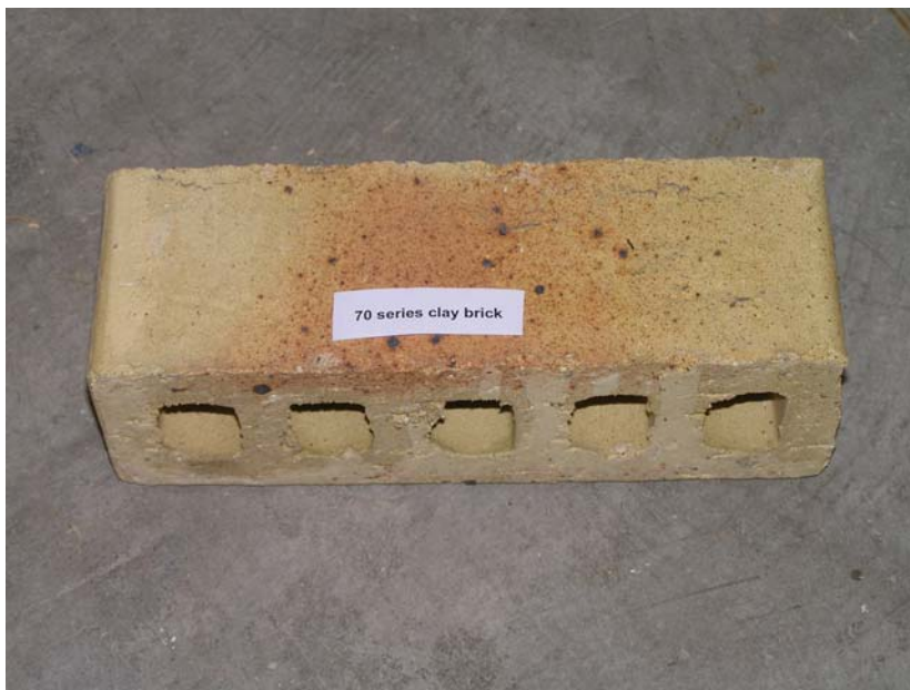
Figure 1: 70 series clay brick with holes
