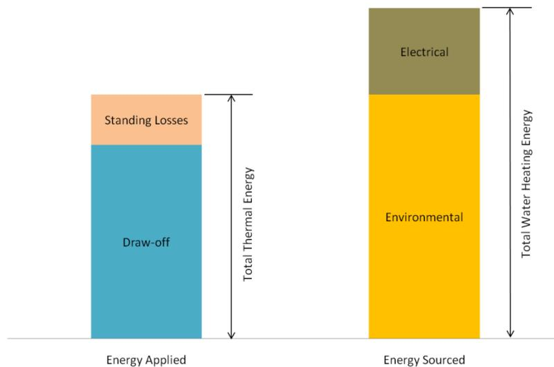
**Figure 3. An example of the energy balance of a HPWH system**
