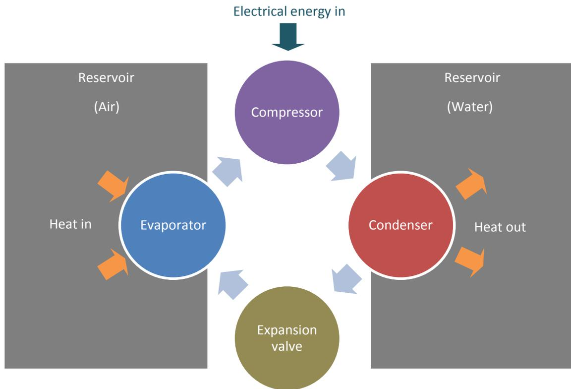
**Figure 1. Heat pump thermodynamic cycle**
