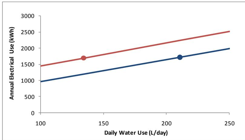
**Figure 5. Example of the performance of two HPWH systems**
