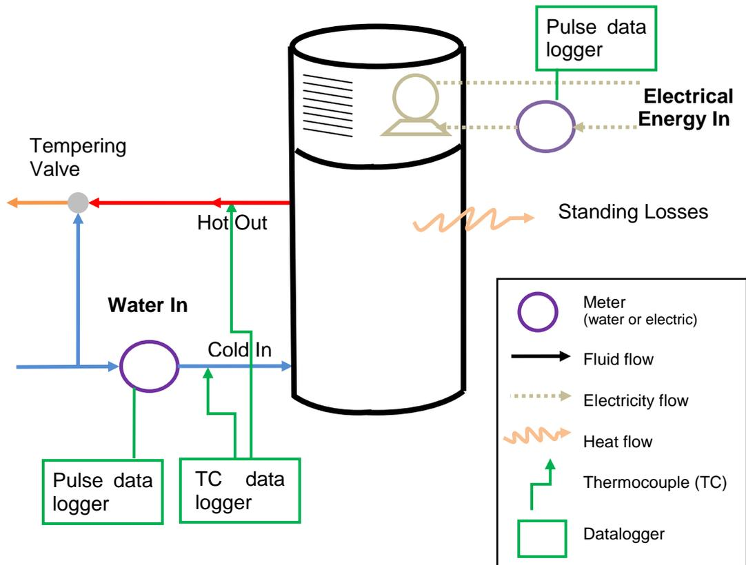
Figure 4. Monitoring arrangement for each HPWH
