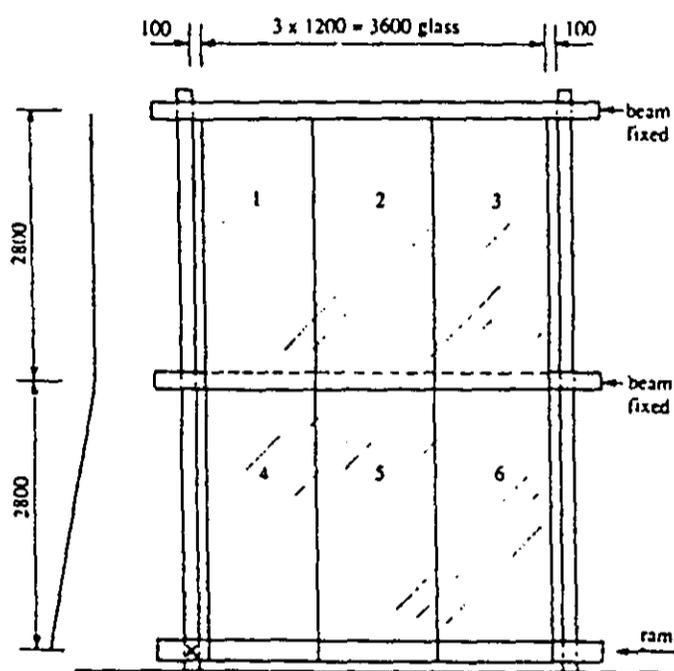
Figure 3: Double storey specimen with zero adjacent interstorey drift (configuration zd).
