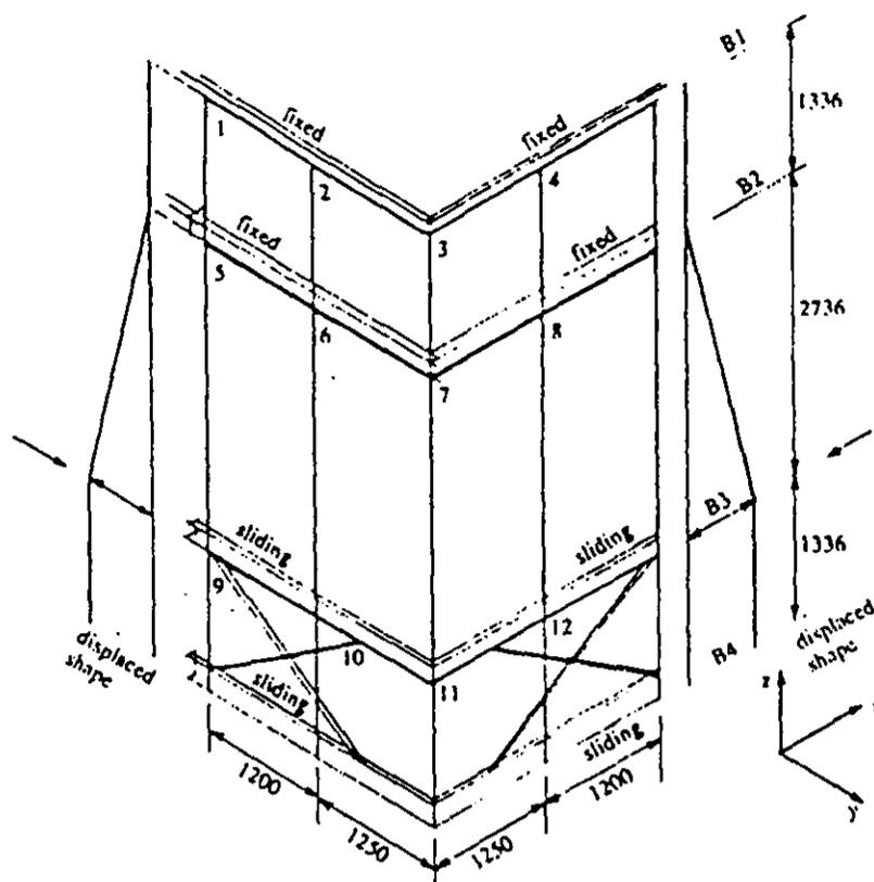
Figure 5: Corner specimen with zero adjacent interstorey drift (configuration cf).
