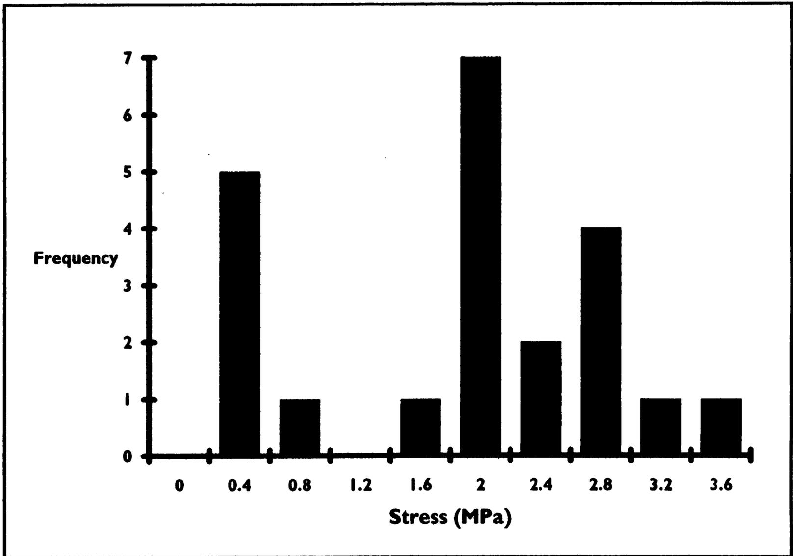
Figure 3. Bi-modal distribution of shear failure stresses for adhesive 5 conditioned from 95% to 65% RH
