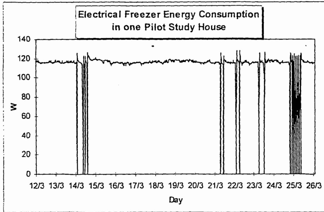
FIGURE 7: Energy consumption of an old chest freezer. The cycling process was obviously faulty. It has not yet been established whether the fault was caused by a defect in the thermostat or other faults.
