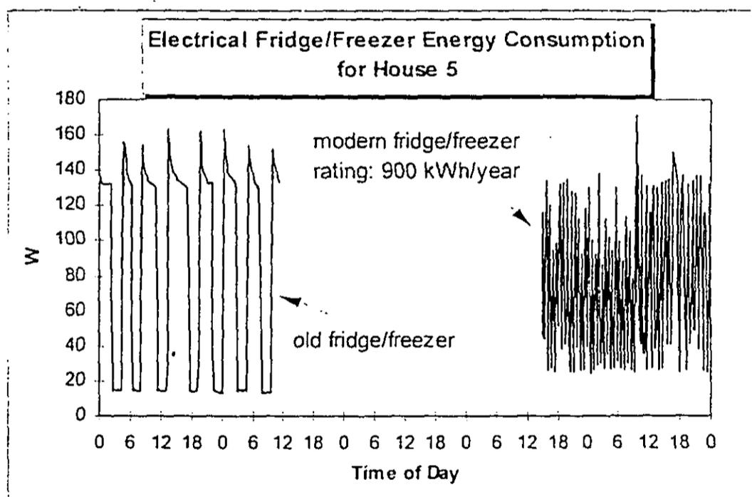
FIGURE 6: Energy consumptions of an old and a new fridge/freezer of similar sizes (260l fridge, 110l freezer volume). The old model uses approximately 30% more energy than the newer model.
