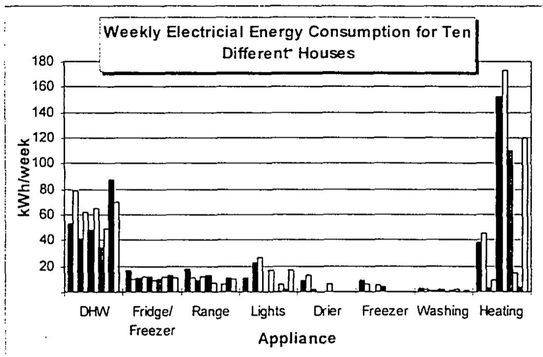
FIGURE 3: Comparison of weekly electrical energy consumption of the ten houses monitored in Wanganui. The largest variation in weekly electrical energy consumption appears for heating energy use. The four largest energy uses are in houses with night-store heaters.
