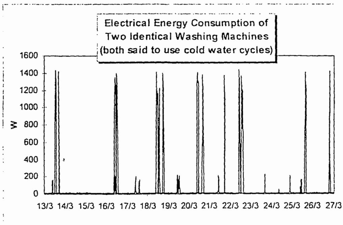
FIGURE 8: Energy consumption profiles of two washing machines with similar specifications. Both operators stated that they would apply cold water washing cycles.
