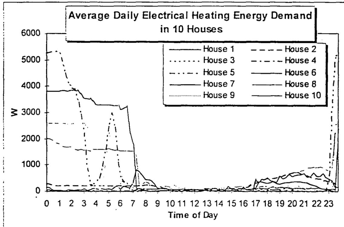
FIGURE 5: Average daily electrical heating energy demand in ten houses. There is a clear distinction in the demand pattern between houses with night-store heaters and those without. The heating energy use in the houses with night-store heaters is significantly higher than in those without. In two of the houses the night-store heater has to be recharged a second or even a third time during the night period.
