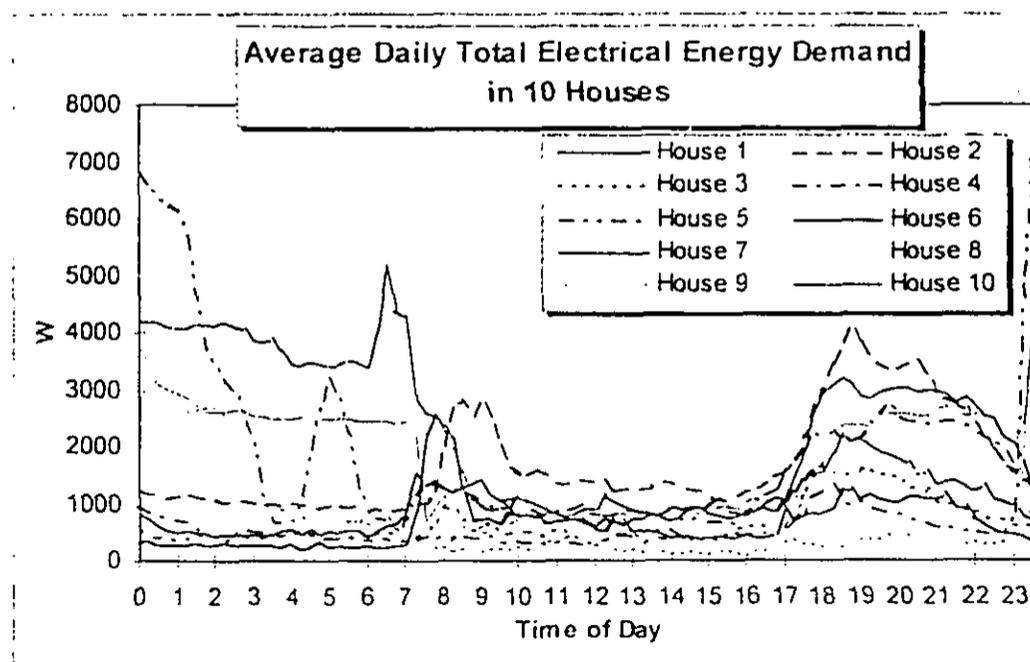
FIGURE 4: Comparison of average total demand for 10 houses in Wanganui. The relative variations between the houses are significant. The typical night-store demand pattern is visible for houses 5, 6, 7 and 10. House 9 uses night rate electricity for hot water heating.
