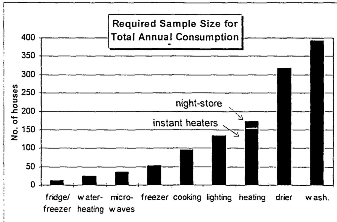
Figure 2: Required sample size for the total annual electricity consumption with an acceptable error of 10% and a confidence interval of 90%. The large sample size in the 'washing' category is caused by the combination of washing and drying in some of the current houses
