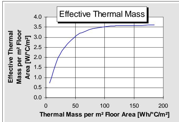
Figure 2: Effective thermal mass as a function of total thermal mass
