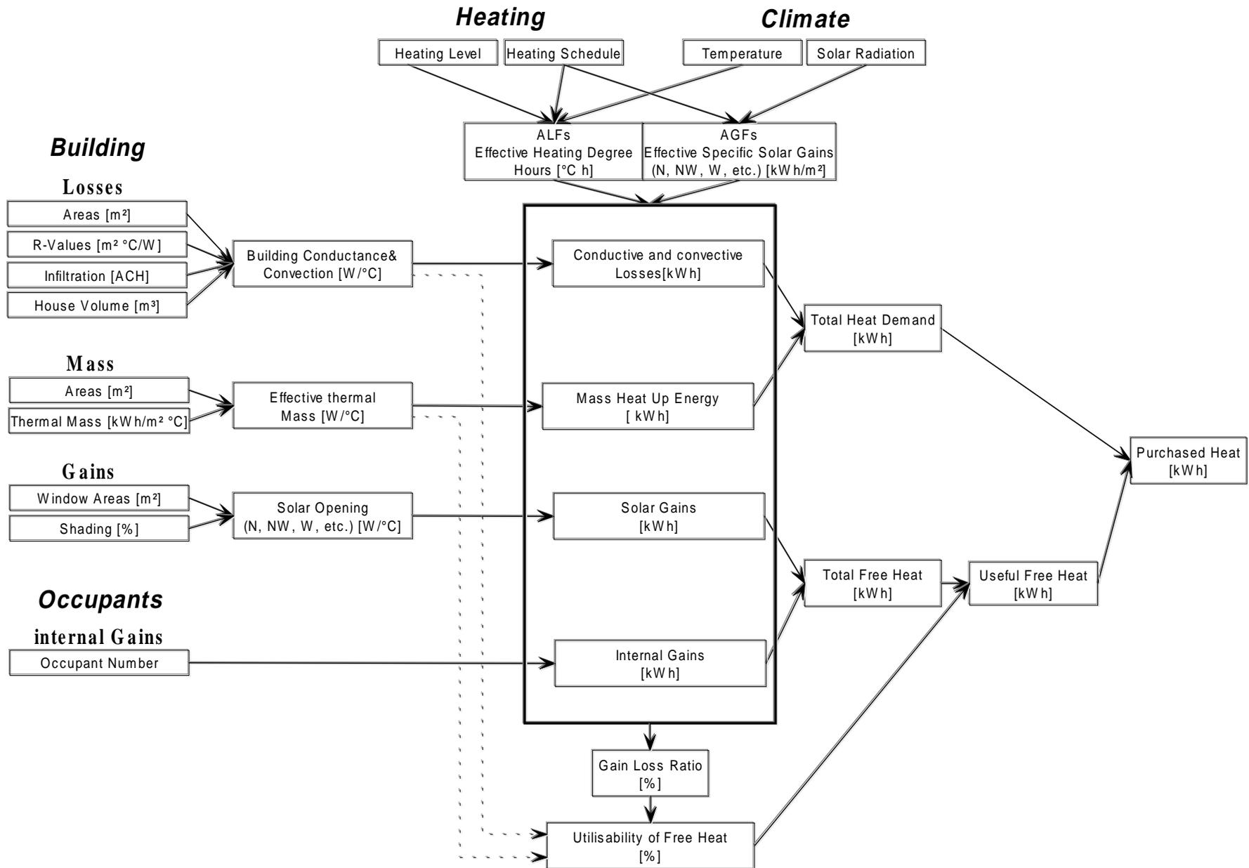
Figure 1: Structure diagram of the ALF 3 calculation steps
