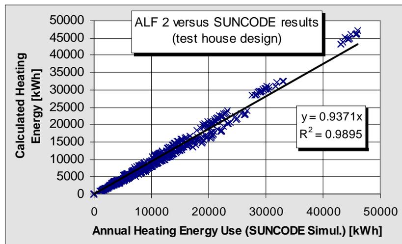
Figure 5: Comparison of SUNCODE and ALF 3 energy calculation for a test house design
