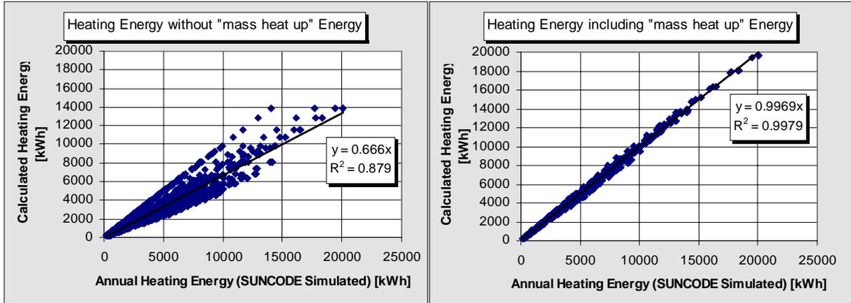
Figure 4: Calculated heating energy versus SUNCODE simulated energy. The left graph shows the comparison without taking account of the energy required to heat up thermal mass in the building, the right graph shows the comparison of the calculation which does account for mass heat up energy.
