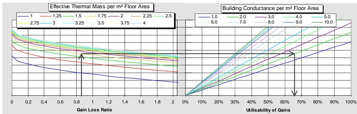
Figure 3: Determination of the utilisability of heat gains: 1. Calculate and select Gain/Loss Ratio (left graph), 2. Determine vertical intersection with Effective Thermal Mass (left graph), 3. Determine horizontal intersection with Building Conductance (right graph), 4. The resulting ordinate value of the right graph is the utilisability of the gains
