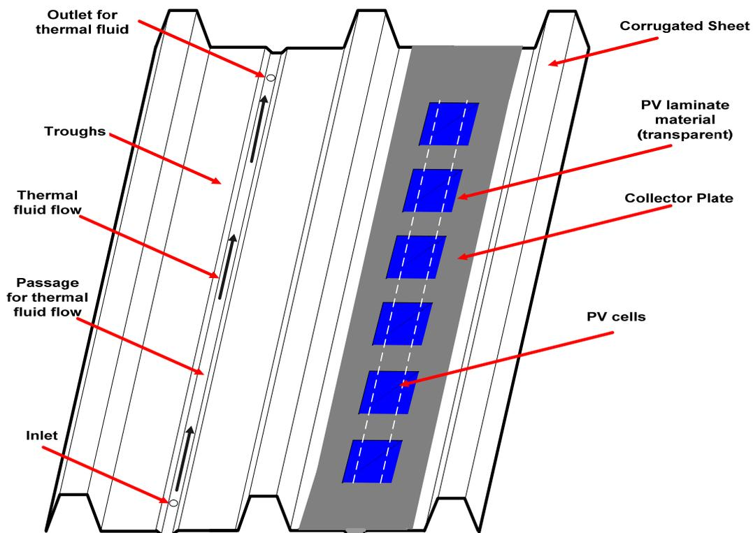
**Figure 1:** Schematic view of BIPVT product
