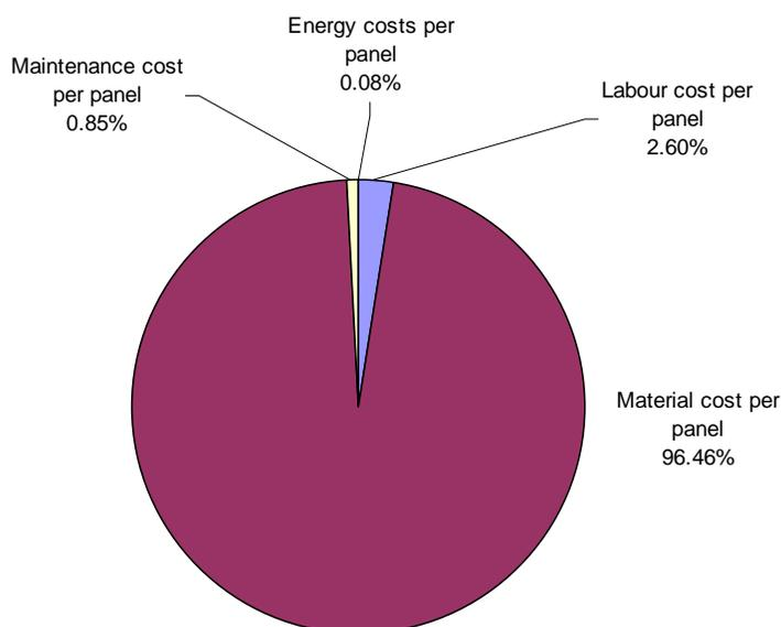
**Figure 4.** Materials, maintenance, labour and machine costs per panel
