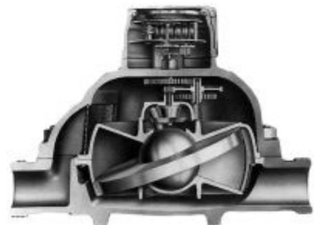
**Figure 7: Nutating disk meter**
