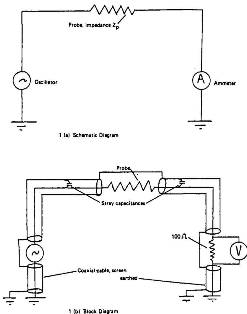
Figure 1. Diagrams of the ac impedance probe measuring circuitry
