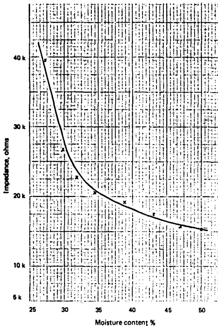
Figure 2. AC impedance at 5°C — typical single probe
