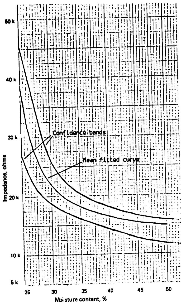
Figure 4. AC impedance at 5° C — all probes
