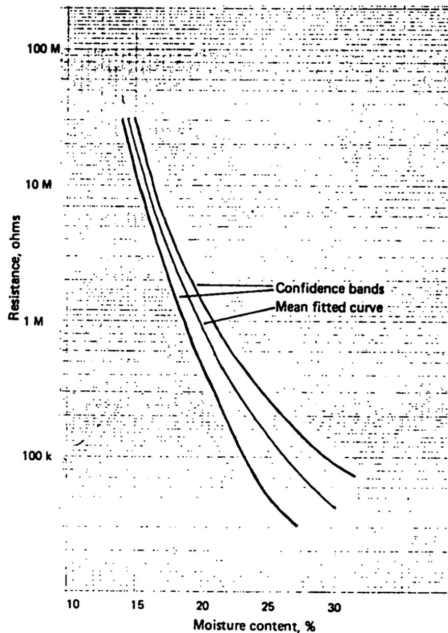
Figure 7. DC resistance at 20° C — all probes
