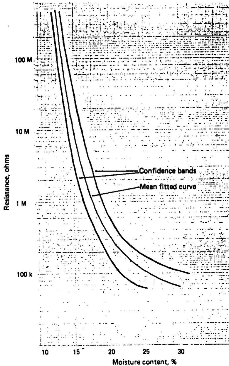
Figure 5. DC resistance at 5° C — all probes
