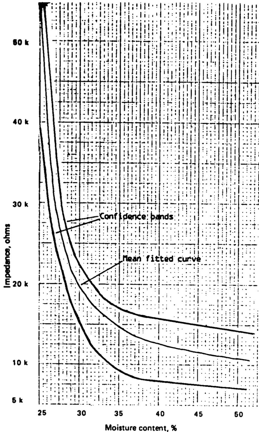
Figure 6. AC impedance at 20° C — all probes
