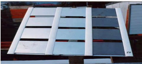
Figure 1: General exposure rack stamped with identification numbers on the skyward faces and the racks were assembled at BRANZ, prior to dispatch to the sites.
