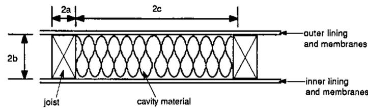
Fig. 3. Diagram of the structure type modelled.
