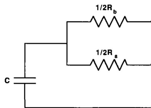
Fig. 2. Electrical circuit analogue for hygroscopic materials.
