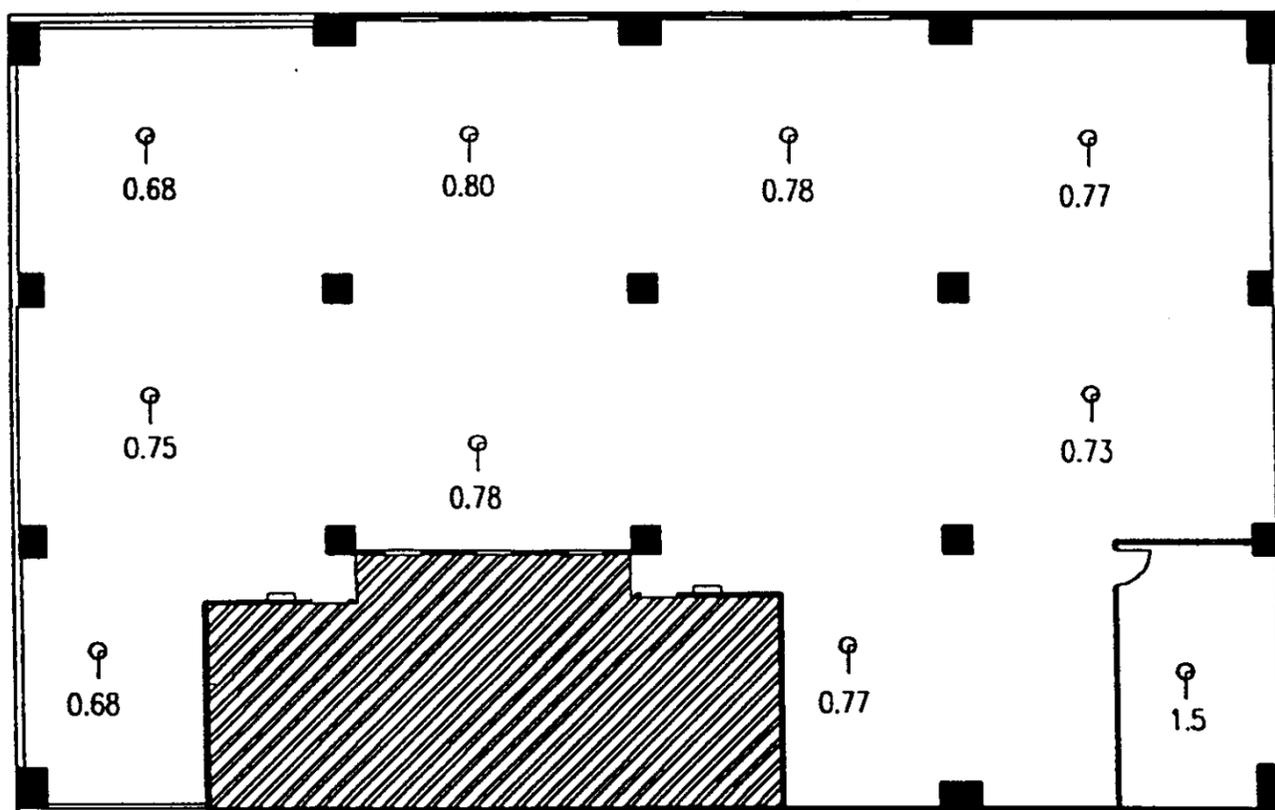
Figure 5: Local mean age-of-air data (in hours) for building B second floor
