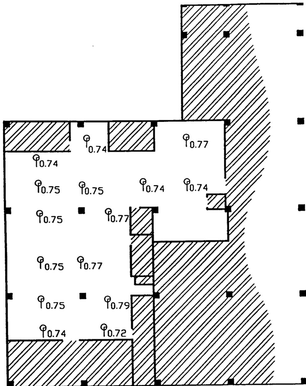
Figure 5: Local mean age-of-air data (in hours) for building A middle floor.
