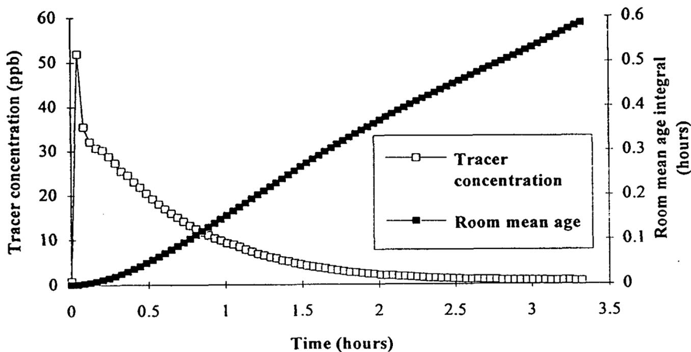
Figure 3: A typical tracer concentration record and developing room mean-age integral.
