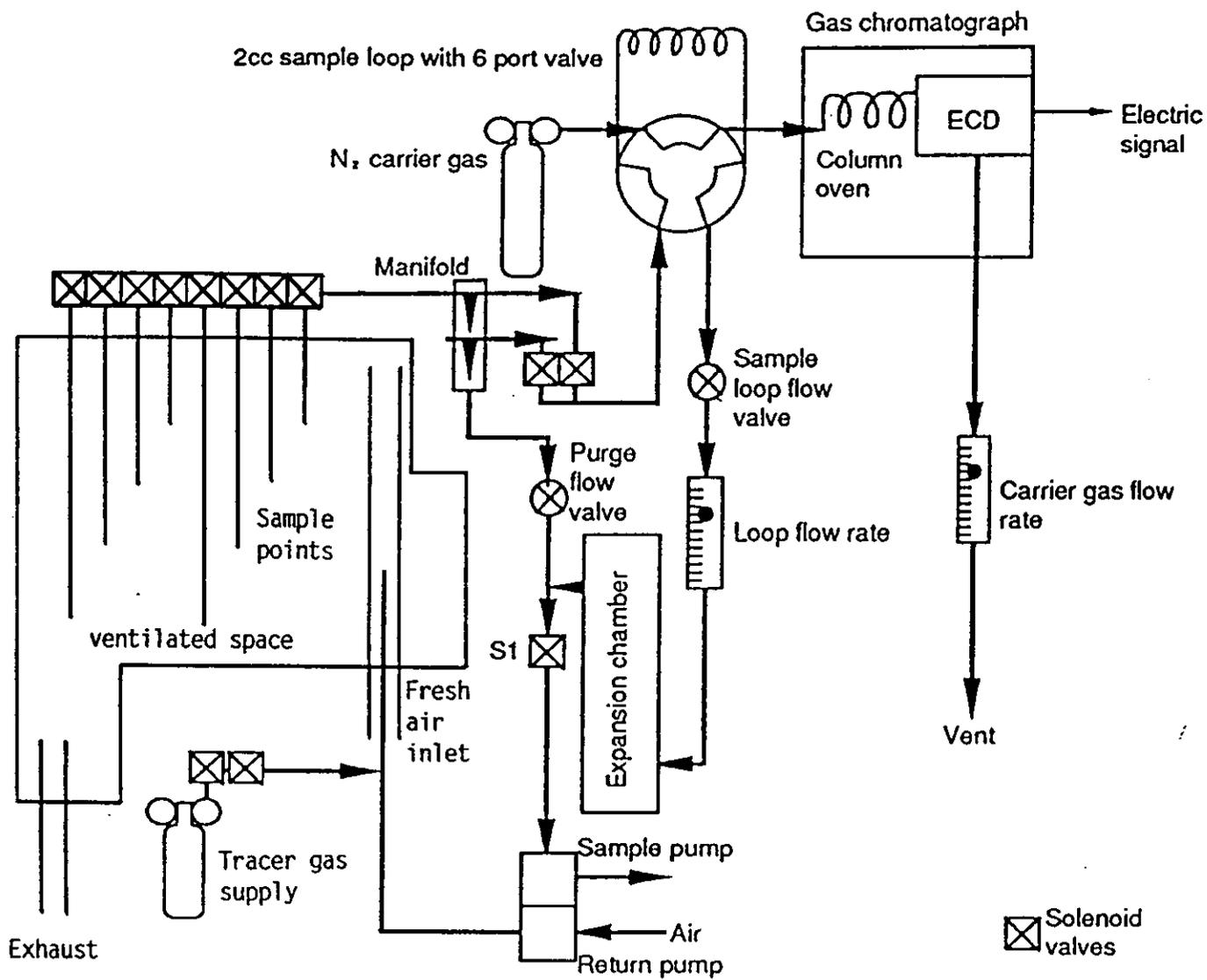
Figure 1: Tracer gas delivery and detection system for pulse local mean-age measurements.
