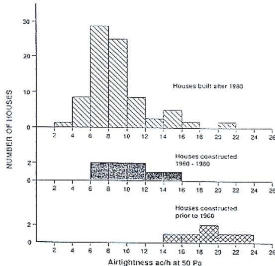
**Figure 2: Histogram of air change rates at 50 Pa for 40 New Zealand houses (Bassett 1992)**
