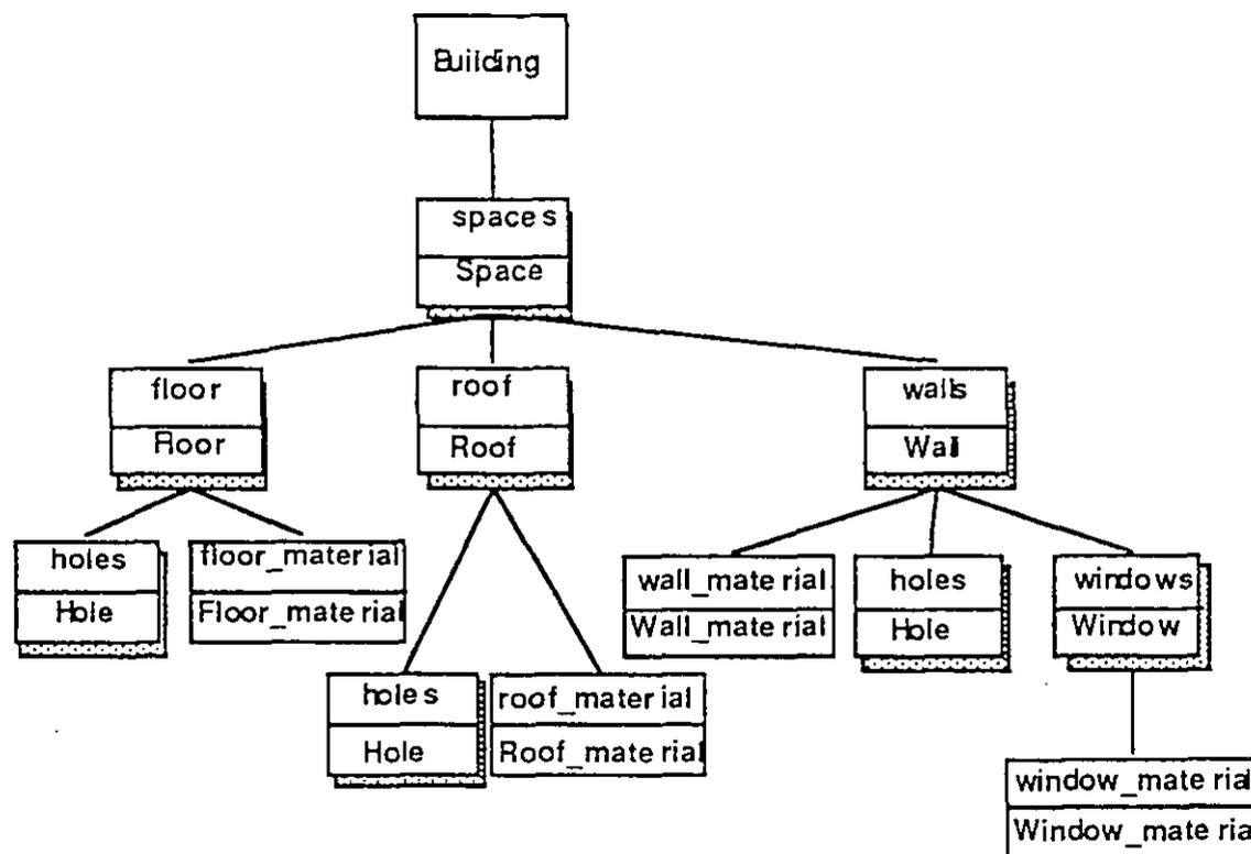
Figure 1: Class structure diagram of ThermalDesigner building model
