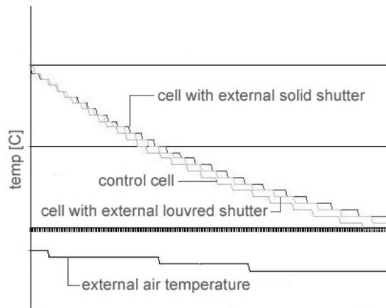
Figure 4: Internal temperature of test cells overnight
