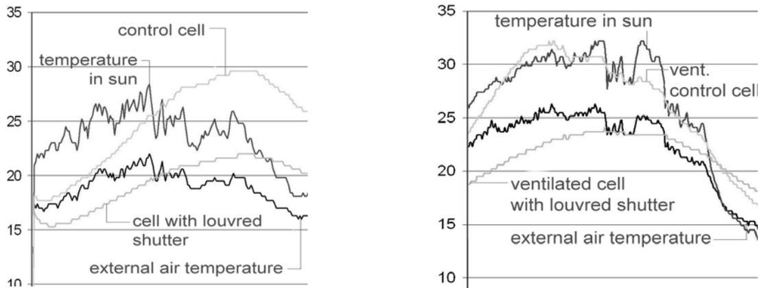
Figure 8 and figure 9: test cells with louvred shading: with and without ventilation
