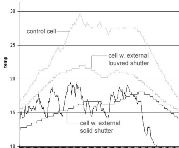
Figure 5: Internal temperatures in shaded test cells (external air temperature shown in black)
