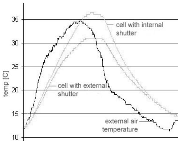
Figure 7: Internal shading compared with external shading
