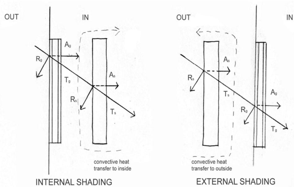
When solar radiation hits the external shading device, only the transmittance portion of the solar radiation incident on the shading system is transferred to the glazing.
