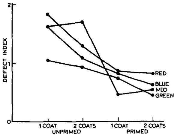
Figure 4. Average defect indices for the four brands of micaceous iron oxide latex paints (the results for the other colours of the same brands are also shown)
