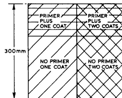
Figure 2. Painting scheme for galvanised steel panels
