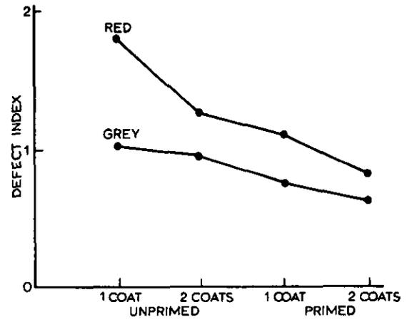
Figure 5. Average defect indices for the three brands of grey paint (the results for red paints of the same brands are also shown)
