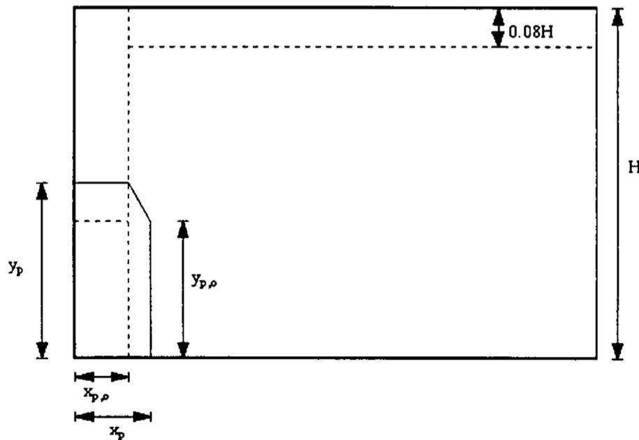
Figure 2: Wall ignited; pyrolysis front has not reached the ceiling
