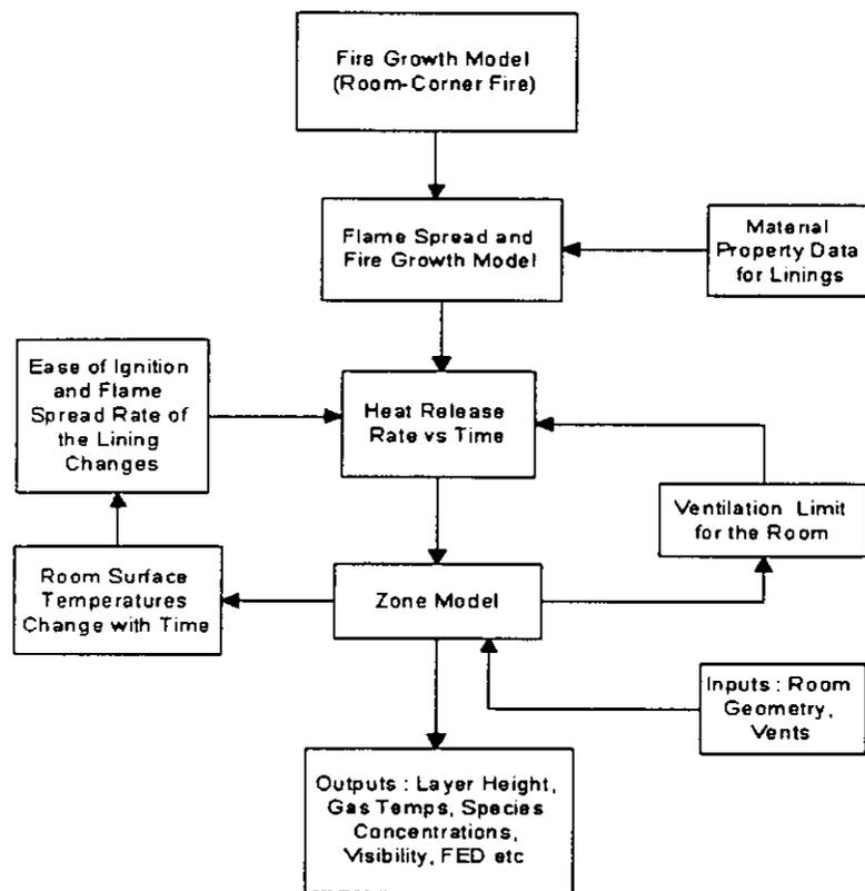
Figure 1: Structure of *BRANZFIRE* Model
