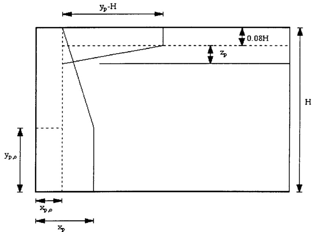
Figure 3: Wall ignited; pyrolysis front has reached the ceiling
