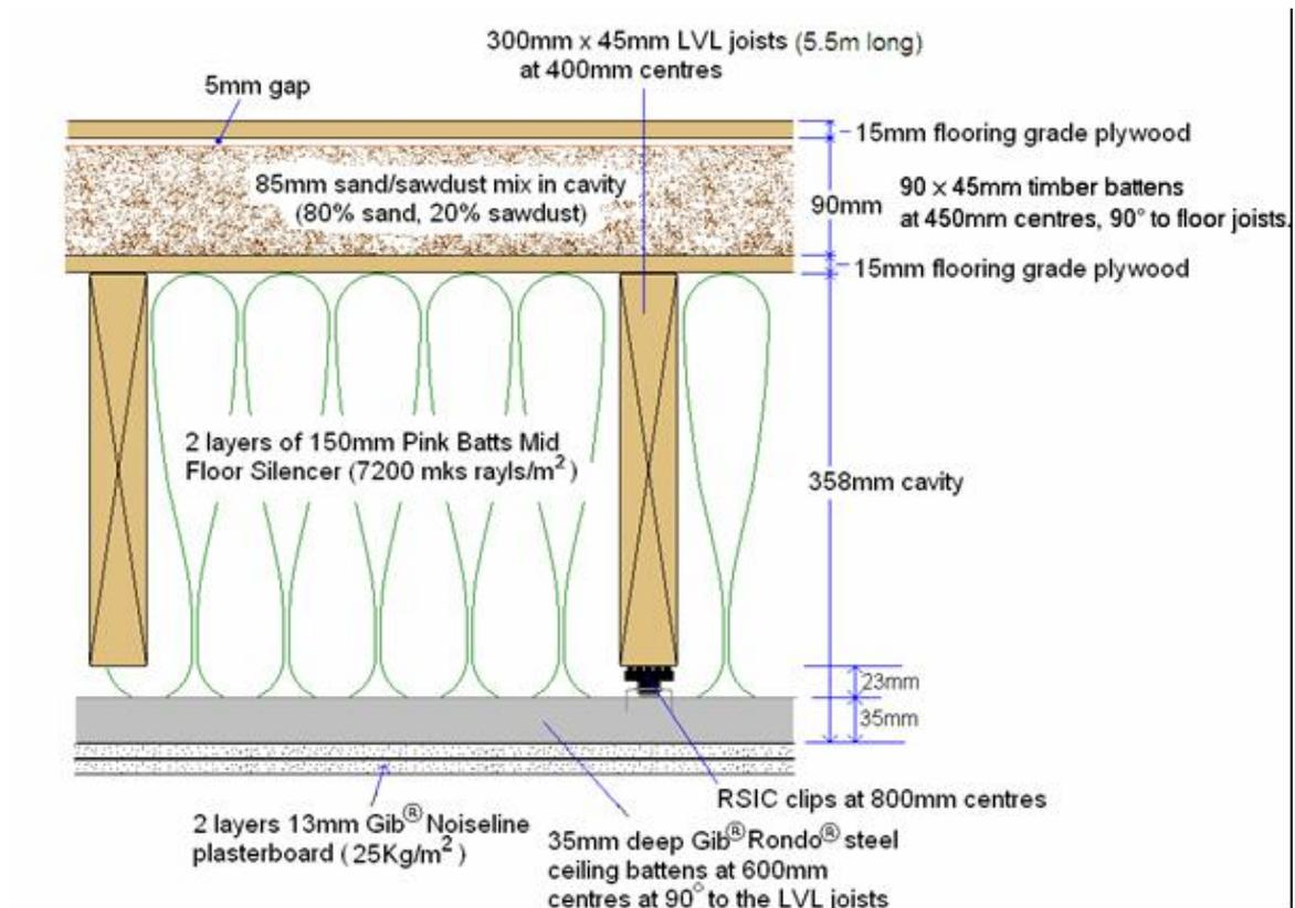
Figure 5. Sand-filled floor.
