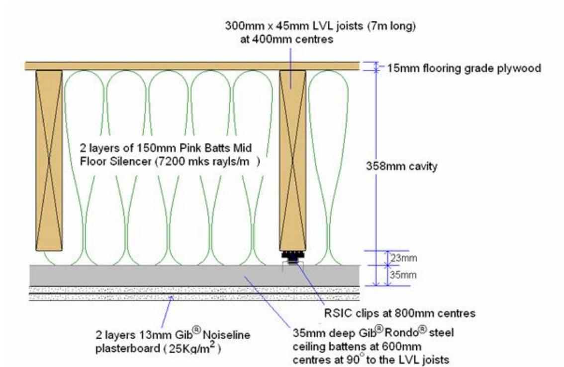
Figure 2. Basic, timber-framed intertenancy floor.
