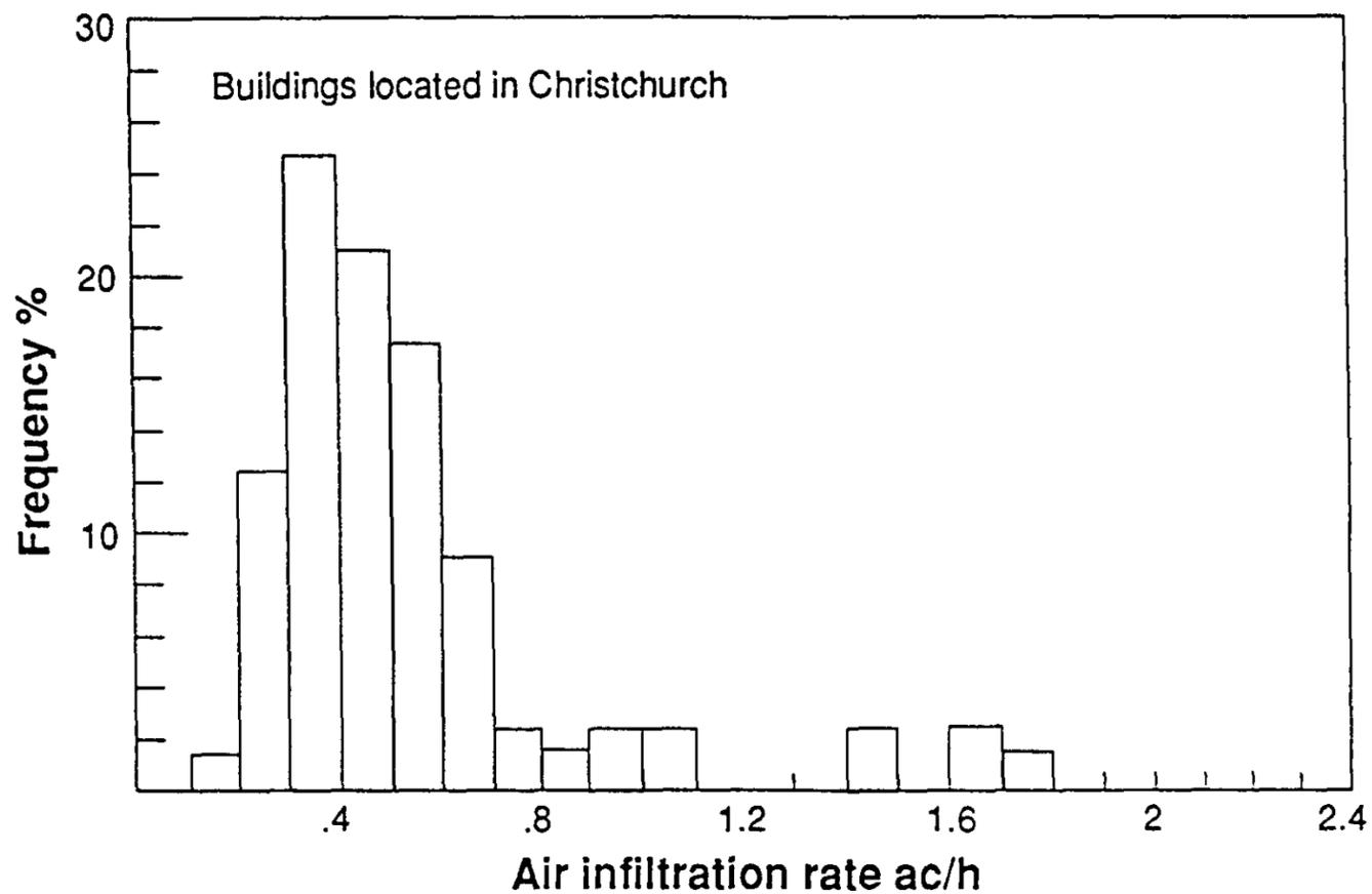
Figure 6: Mean winter infiltration rates for buildings of all airtightness levels located in the Christchurch climate.
