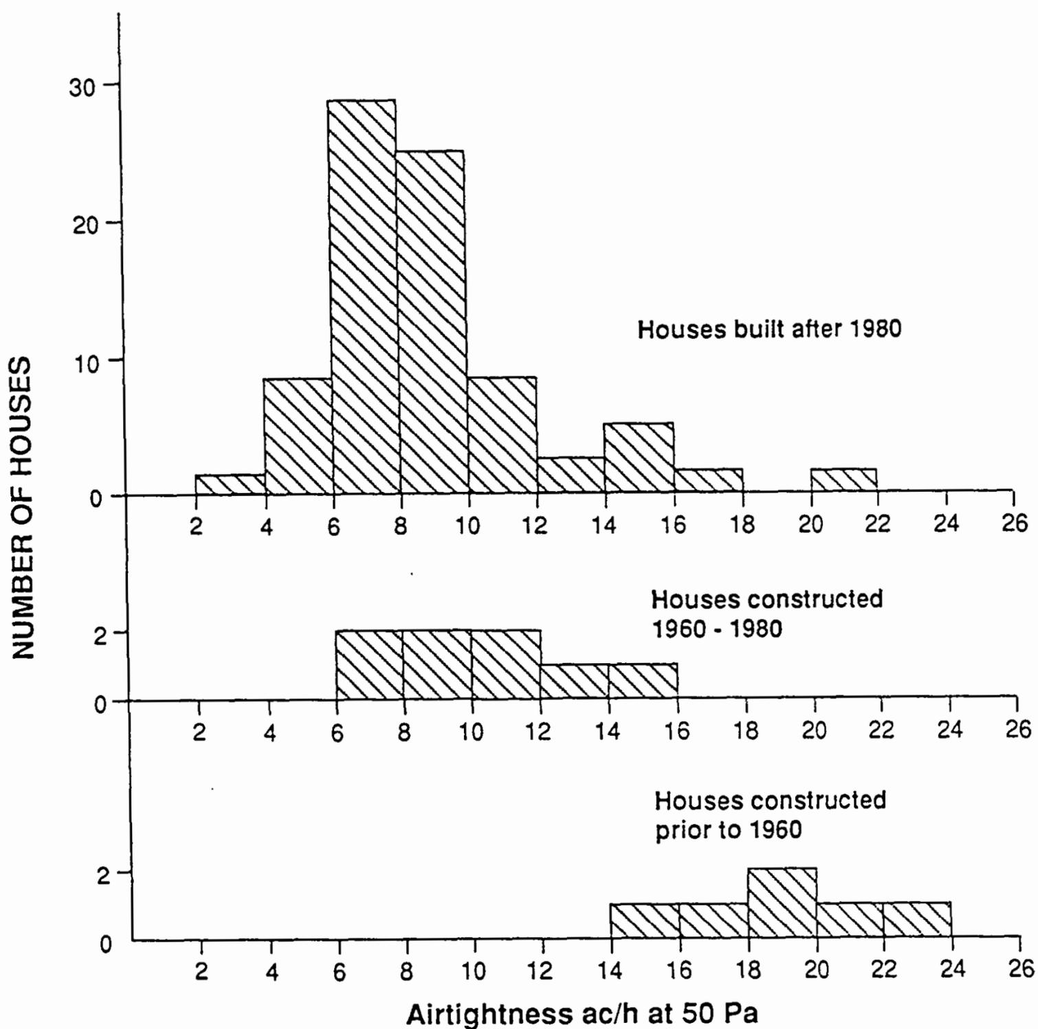
Figure 3: Airtightness of New Zealand houses measured at 50 Pa
