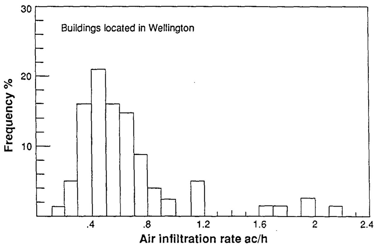
Figure 5: Mean winter infiltration rates for buildings of all airtightness levels located in the Wellington climate.
