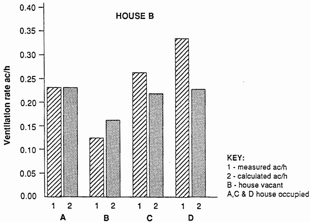
Figure 8: Ventilation rates measured in house B compared with calculated air infiltration for the same period.
