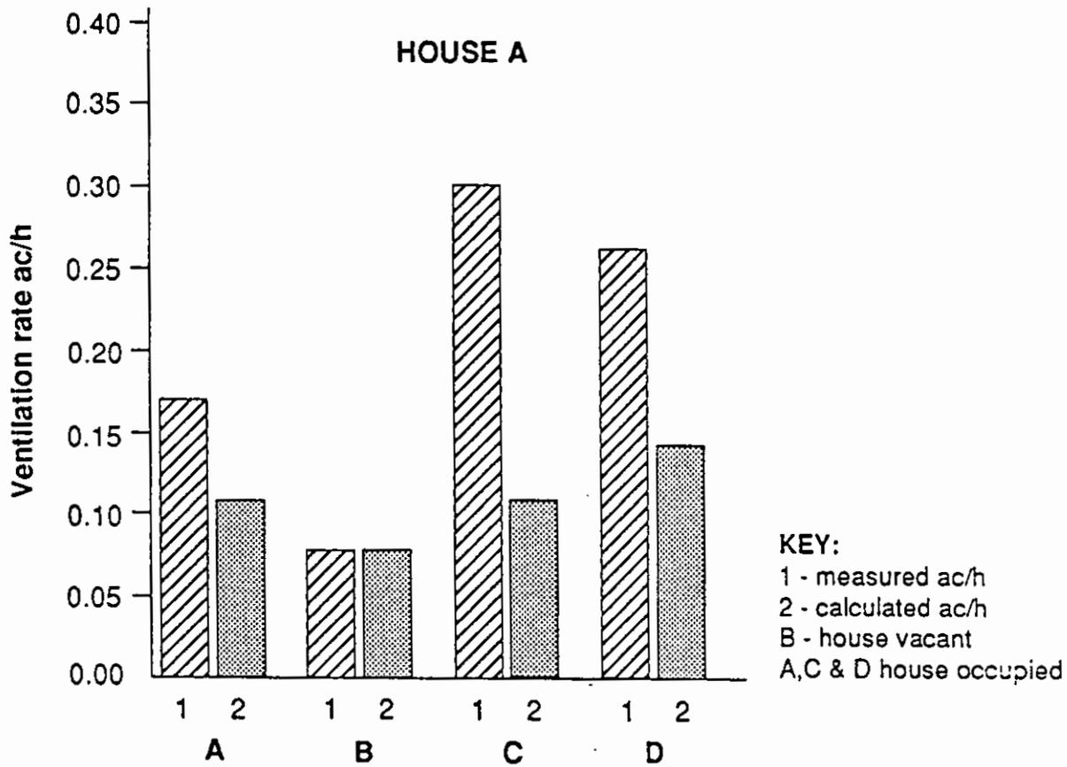
Figure 7: Ventilation rates measured in house A compared with calculated air infiltration for the same period.
