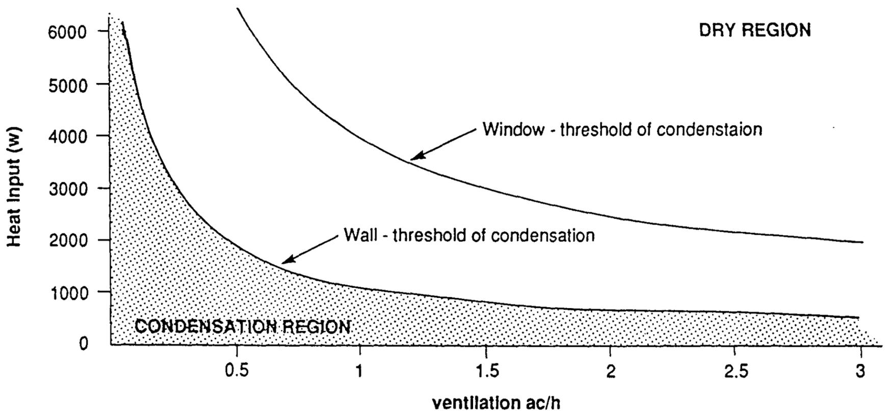
Figure 1: Condensation threshold curves for an insulated wall and a single glass window
