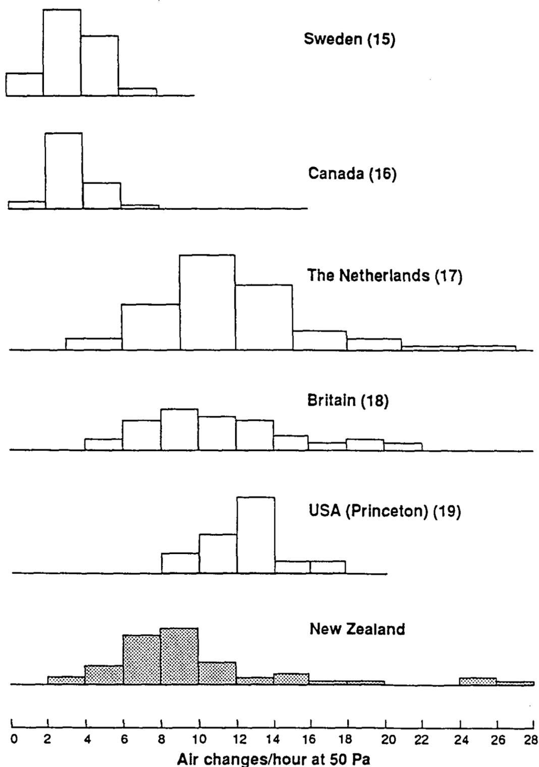
Figure 4: Relative airtightness of houses measured at 50 Pa
