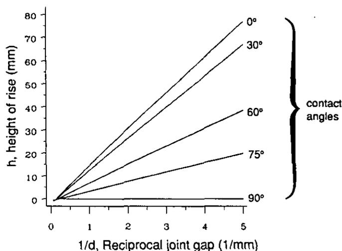
Fig. 2. Height of capillary rise of water vs reciprocal joint gap, for various contact angles.
