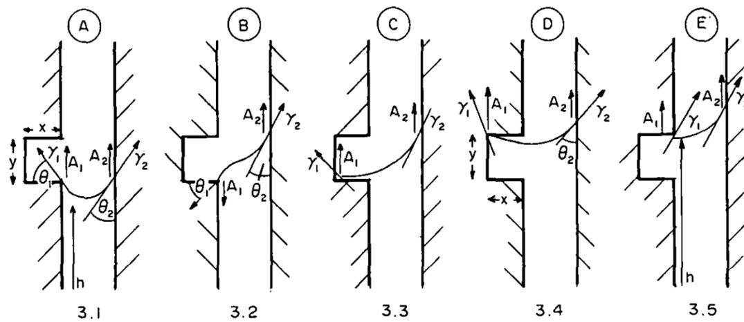
Fig. 3. Meniscus behaviour at a weathergroove.
