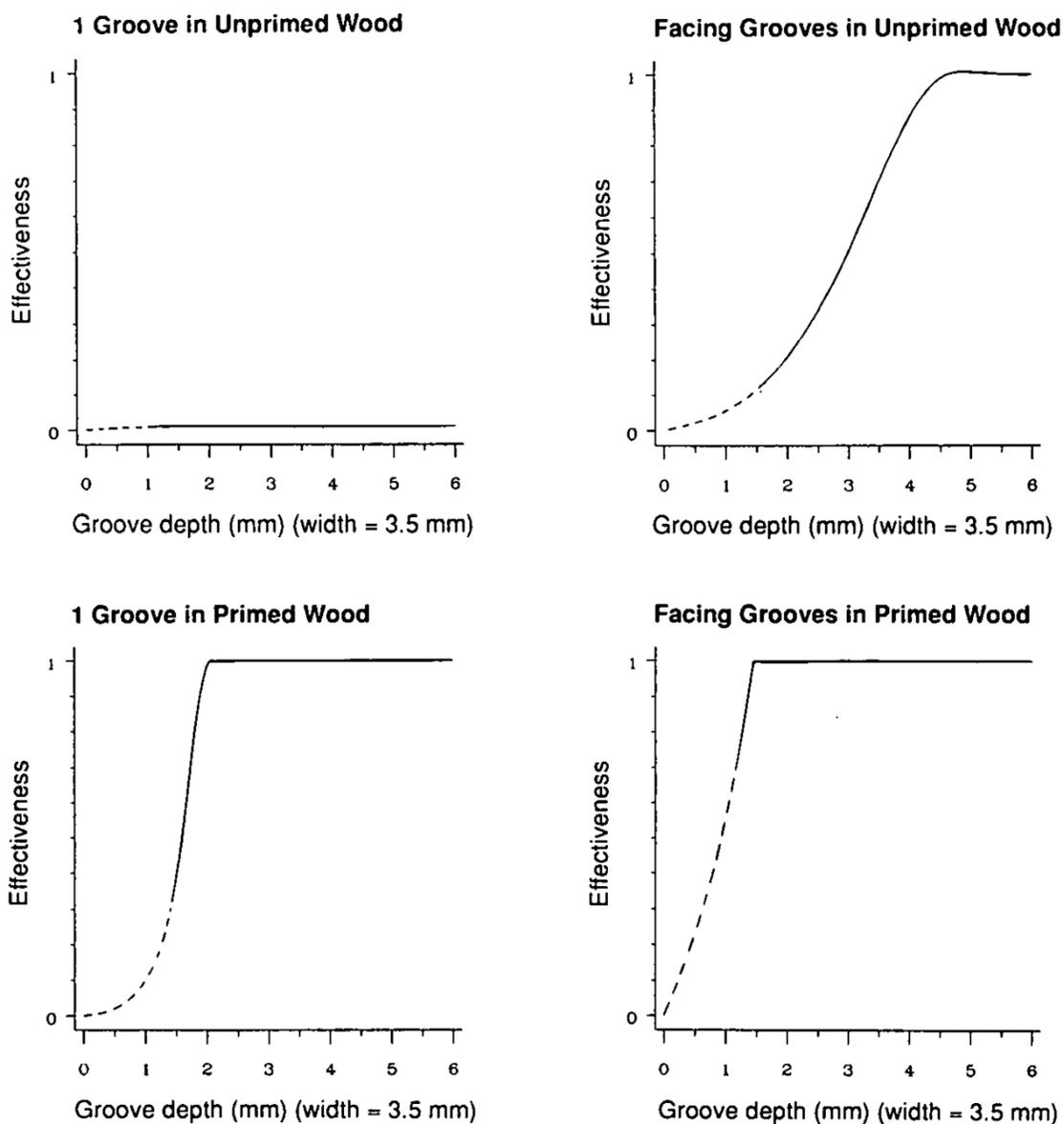
Fig. 6. Graphs of critical sizing of weathergrooves. Data taken with height of groove above free liquid surface  $h = 30$  mm in unprimed wood,  $h = 10$  mm in painted wood, (typical for weatherboards). Width of groove is nominally 3.5 mm (due to width of typical saw-blade) and joint is tight.
