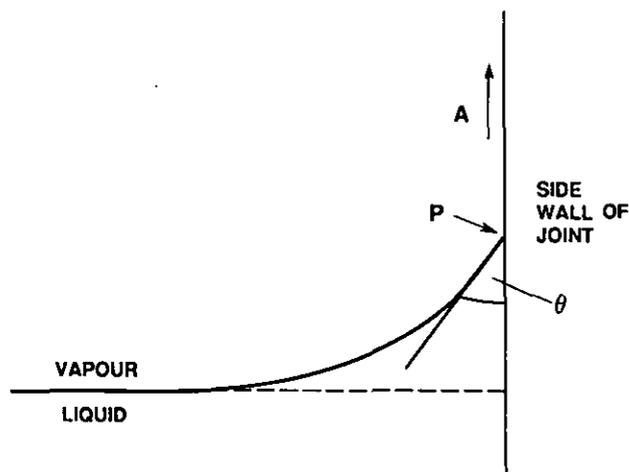
Fig. 1. The capillary curve.
