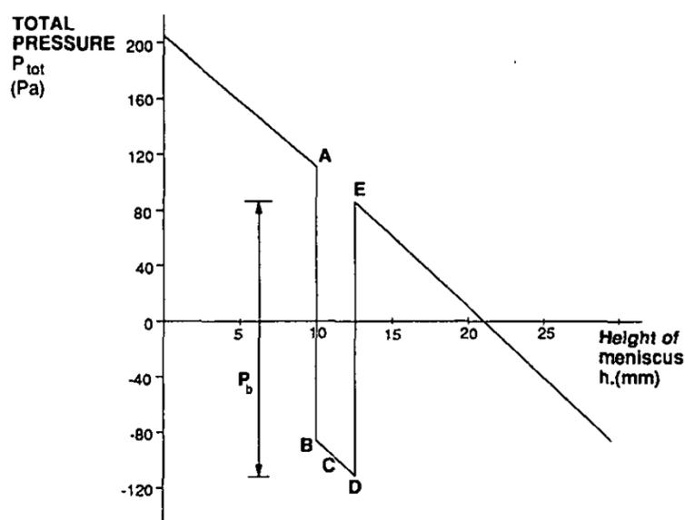
Fig. 4. Graph of  $P_{tot}$  for a joint 0.4 mm wide. An applied pressure exceeding  $P_b$  will provide enough pressure to allow breaching, and prevent the graph going negative. Weathergroove is 3.0 mm deep  $\times$  2.5 mm, between  $h = 10$  and 12.5 mm.
