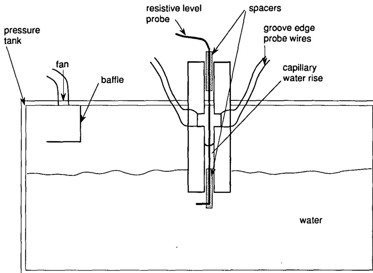
Fig. 5. Laboratory pressure tank and sample joint.
