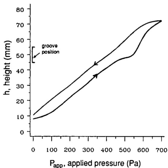
Fig. 7. Hysteresis plot of height vs applied pressure. Water driven into a simulated horizontal lap joint gap of 0.9 mm, to display the effect of a groove between  $h = 45$  and 55 mm, in a pressure driven system.
