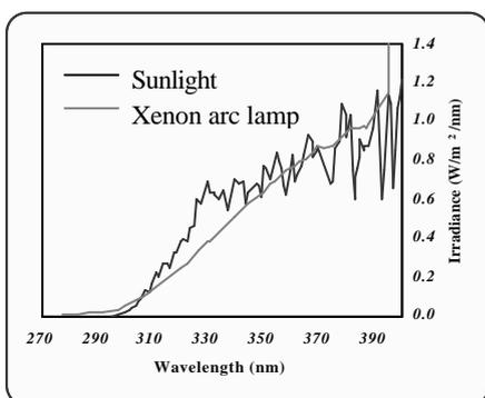
**Figure 3. Irradiance output from xenon arc lamp**
