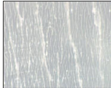
**Figure 5. Microcracking of UV exposed polypropylene**
